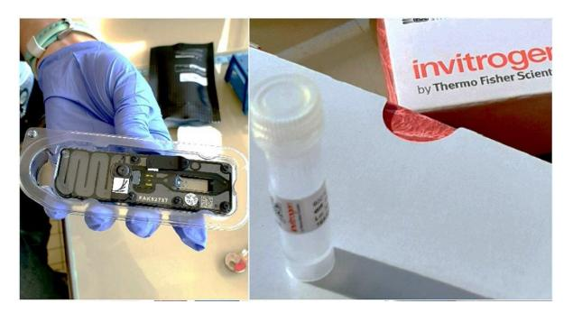
Figure 3.3: The right part of the figure represents a test tube which contains thousands of copies of an ordered synthetic DNA sequence. The left part represents a flowcell which is a consumable that is used on the MinION sequencer to sequence DNA. The experiments were performed at INRAE STLO Rennes.
