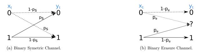
Figure 4.3: Examples of standard telecommunication channels
