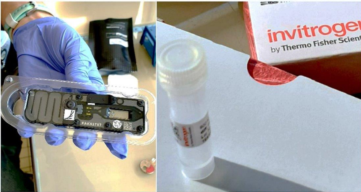
Figure 3.3: The right part of the figure represents a test tube which contains thousands of copies of an ordered synthetic DNA sequence. The left part represents a flowcell which is a consumable that is used on the MinION sequencer to sequence DNA. The experiments were performed at INRAE STLO Rennes.
