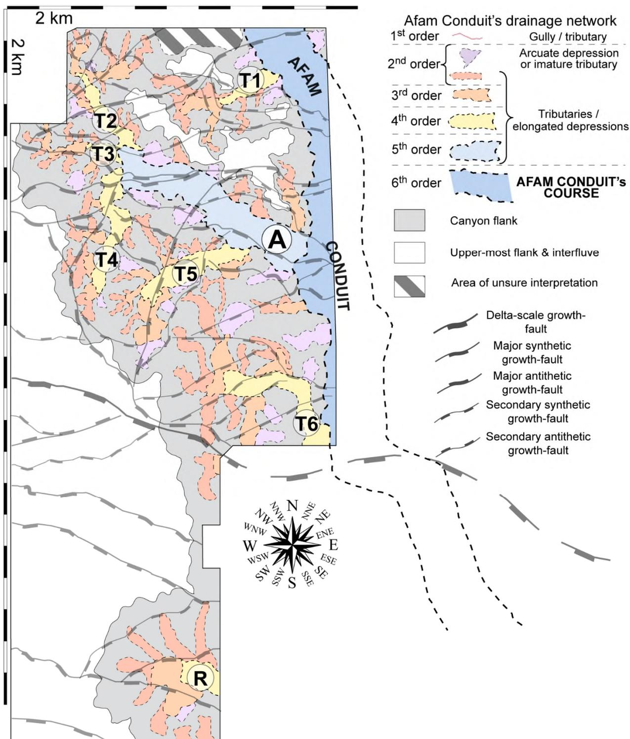
Figure V-7. Interpreted structural scheme of the northern study area, superimposed on the interpreted Afam drainage network using the Strahler's (1957) method. The 1<sup>st</sup> order tributaries has not been interpreted due to the poor resolution of the 3D seismic data of the northern seismic block and due to the methodology used for the of interpretation of the IAS, using only time slices.
