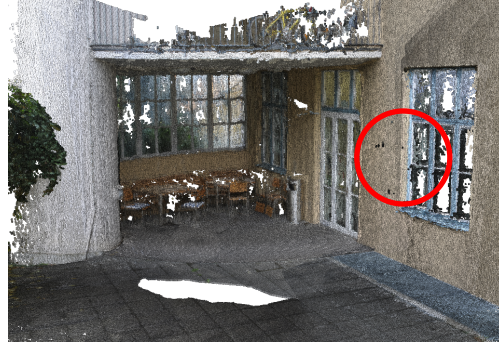
(b) Terrestrial MVS Point Cloud
