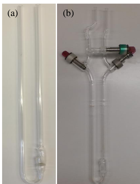
Figure 2.21 The reactor used for various pretreatments. (a) U-shape reactor equipped on catalytic setup, (b) U-shape reactor with three valves equipped on vacuum line.
