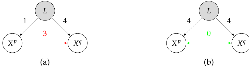
Figure 3.2 – How TCDF deals with hidden confounders. A red edge (a) indicates a wrong causal relation discovered by TCDF, whereas a green double edge (b) indicates that a true causal relation is discovered. Numbers correspond to delays.
