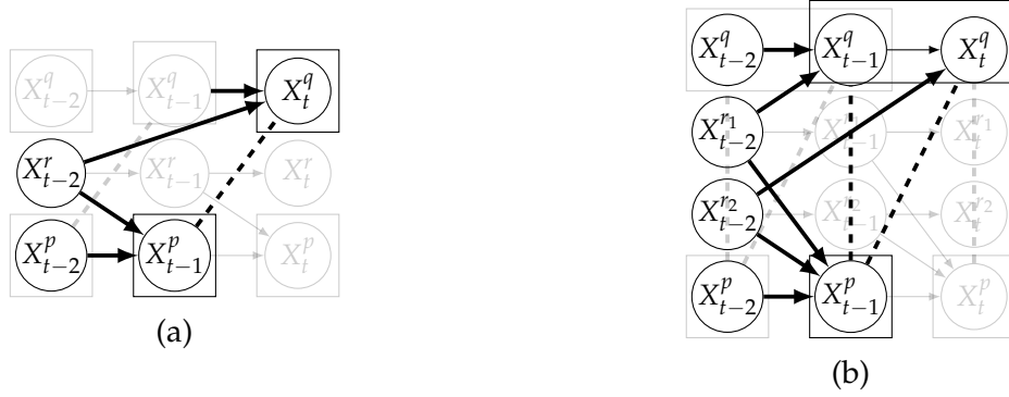
Figure 4.3 – Examples of conditional independence between dependent time series. Dashed lines are for correlations which are not causations, and bold arrows correspond to conditioning variables.
