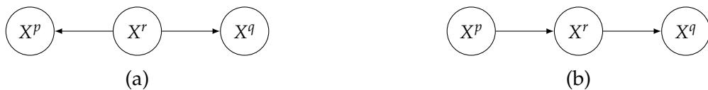
Figure 2.2 – Two causal structures in which X^p is screened off from X^q by X^r .
