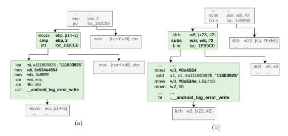
Figure 1.2: CVE-2018-9506 associated CFG for x64 (a) and aarch64 (b)
