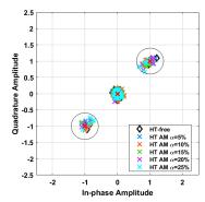
(b) Constellation of the STS<sub>F</sub> preamble using the proposed AM STS HT attack.
