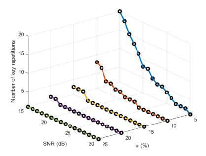
Figure 26: Reliability test for five different modulation amplitudes  $\alpha$  under different SNR scenarios.
