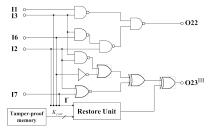
(e) Circuit F<sub>l</sub> after restoring logic in circuit F<sub>f'</sub> for the failing test patterns represented by t<sub>secure</sub>.
