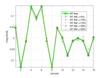
(b) Real (I) part of the HT-free STS<sub>t</sub> and the received STS<sub>t</sub> for different amplitude values in the proposed AM STS HT attack.
