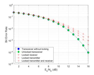
Figure 31: BER measurement results for different configurations.
