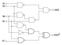
(d) Circuit  $F_{f'}$  after restoring logic in circuit  $F_f$  for all failing test patterns in Fig. 28b except those represented by  $t_{secure}$ .
