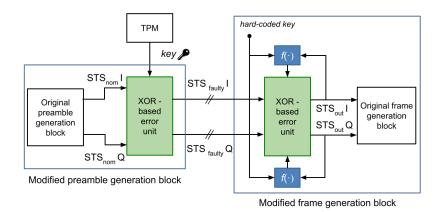
Figure 35: Preamble and frame generation blocks modified for *SyncLock*.
