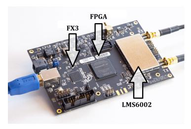
Figure 15: SDR bladeRF board from Nuand.
