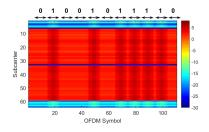
(b) ACE test for an HT-infected transmission based on amplitude modulation at the AFE, like the approach presented in [51]. The HT activity on the payload is identified by the ACE test.
