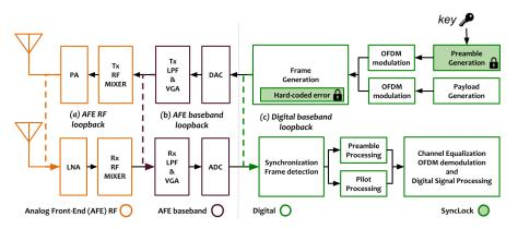
Figure 33: Simplified architecture of a wireless device IC with *SyncLock* embedded.
