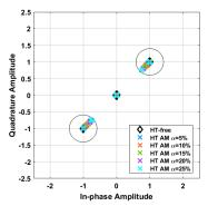
(c) Constellation of the STS<sub>F</sub> preamble using the proposed AM STS HT attack at a high SNR scenario.
