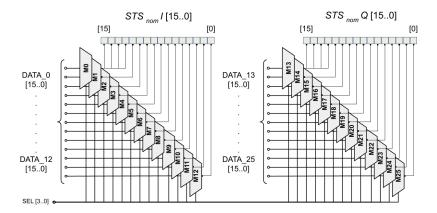
Figure 34: Original preamble generation block with no locking.
