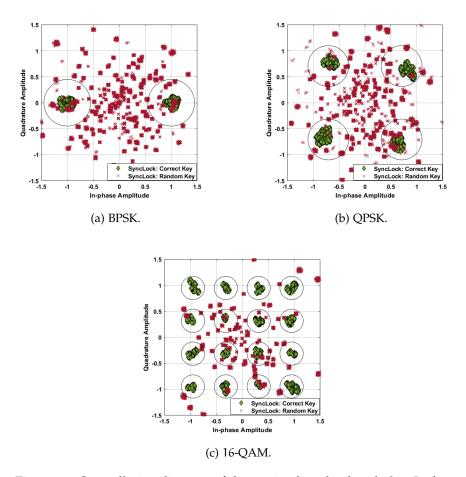
Figure 37: Constellation diagram of the received payload with *SyncLock* embedded.
