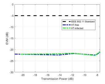
Figure 20: Measured Error Vector Magnitude (EVM) of the transmitted BPSK signal from an AM STS HT-infected device and an HT-free device, along with the IEEE 802.11 standard EVM specification [124].
