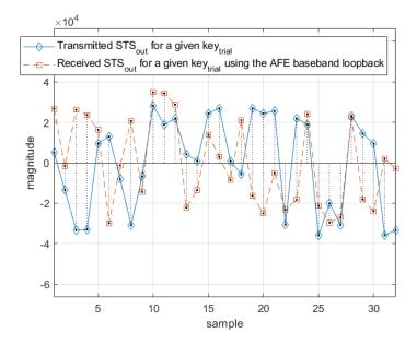
Figure 38: Amplitude values of the first 32 samples of the transmitted and received STS<sub>out</sub> for a given key<sub>trial</sub> using the Analog Front-End (AFE) baseband loopback.
