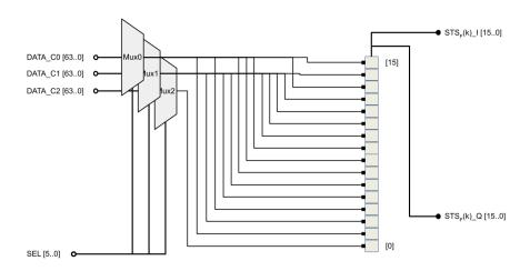
Figure 12: Circuit schematic of the nominal STS block.
