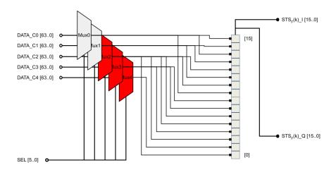
Figure 13: Circuit schematic of the HT-infected STS block.
