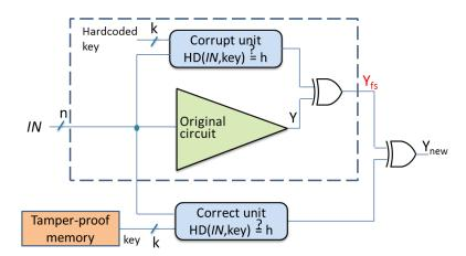
Figure 7: SFLL-hd principle of operation.
