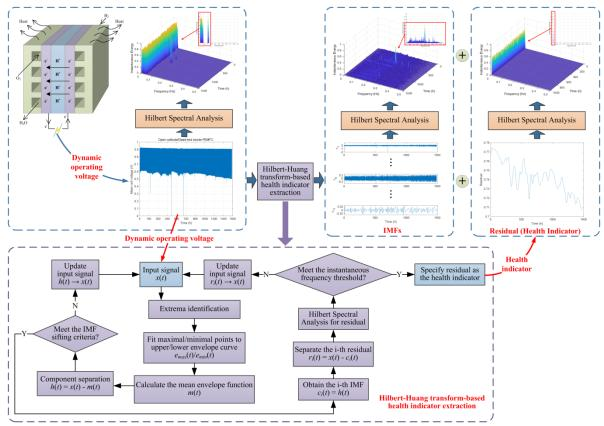
Figure 5.1 Hilbert-Huang transform-based health indicator extraction process.
