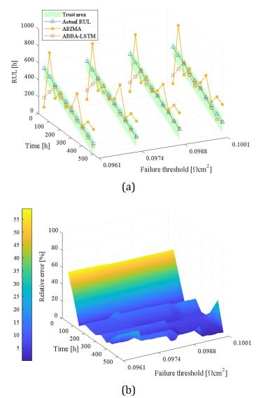
Figure 4.12 For  $HI_1$ , RUL prediction performance and evaluation at different failure thresholds: (a) comparison experiments and prognostics horizon evaluation; (b) relative error of the CFR (0.0961-0.1001  $\Omega$ cm<sup>2</sup>).
