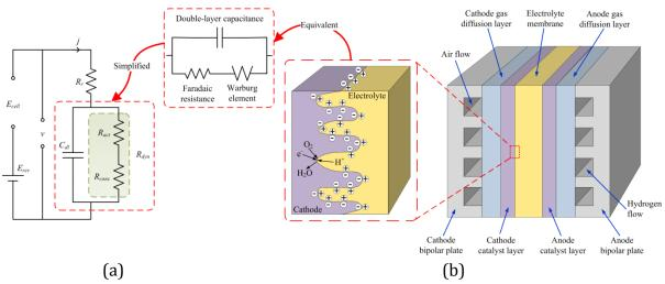
Figure 4.1 PEMFC electrochemical mechanism schematic: (a) equivalent circuit model; (b) physical representation of an electrochemical reaction interface.
