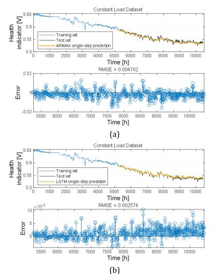
Figure 3.4 Single-step prediction at split point A of constant-load dataset, (a) ARIMAX model; (b) LSTM model.
