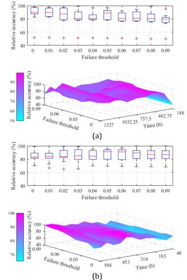
The distribution of RAs at different failure thresholds from: (a) FC-1; (b) Figure 5.10 FC-2.
