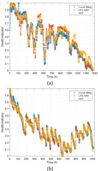
Figure 5.7 Comparison of health indicators extracted based on HHT with the other two methods, for (a) FC-1; (b) FC-2.
