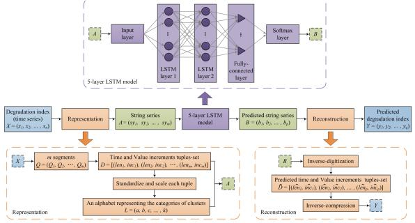
Figure 4.4 Flowchart of the proposed ABBA-LSTM prognostics model.
