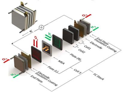
Figure 2.2 Structure diagram of fuel cell stack and components [19].
