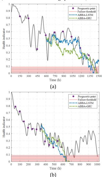
Figure 5.8 Prognostics points set on health indicators, for (a) FC-1, (b) FC-2; Comparison of trends predicted by ABBA-LSTM and ABBA-GRU, (a) from FC-1 at hour 590, (b) from FC-2 at hour 343.
