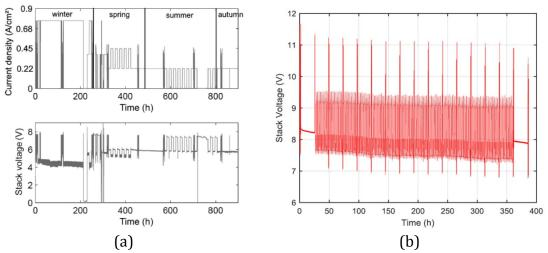
Figure 1.8 Samples of durability tests of PEMFC under variable load conditions: (a) simulated combined heat and power scenario [96]; (b) simulated load dynamic cycling scenario [72].
