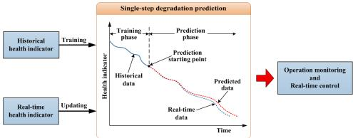
Figure 1.9 Single-step degradation prediction mode.
