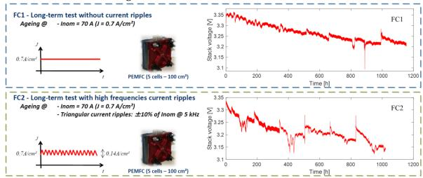
Figure 1.7 Durability test conditions of PHM 2014 challenge: FC1 for constant load; FC2 for quasi-constant load (adapted from [<u>38</u>]).
