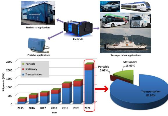
Figure 1.2 Common fuel cell application types and their annual shipments (by megawatt).
