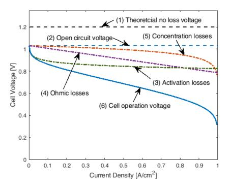
Figure 2.3 Voltage drops of fuel cell.
