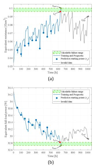
Figure 4.11 Health indicator and failure range for prognostics: (a) equivalent resistance (*HI*<sub>1</sub>); (b) equivalent full-load power (*HI*<sub>2</sub>).
