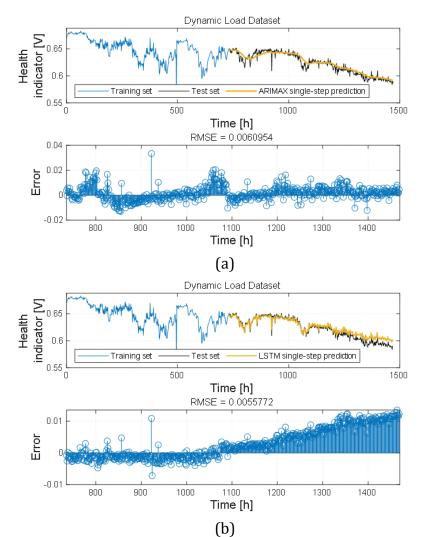
Figure 3.5 Single-step prediction at split point A of dynamic-load dataset, (a) ARIMAX model; (b) LSTM model.
