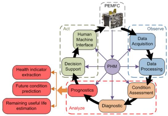
Figure 1.3 Basic architecture of prognostics and health management.
