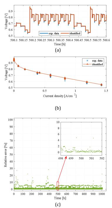
Figure 4.10 Evaluation of dynamic load identification performance: (a) identification of the cell voltage; (b) current density-voltage plot of identification results; (c) relative error of identification results.
