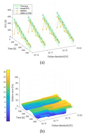
Figure 4.13 For *HI*<sub>2</sub>, RUL prediction performance and evaluation at different failure thresholds: (a) comparison experiments and prognostics horizon evaluation;
