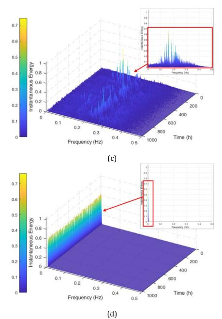
Figure 5.6 For FC-2, (a). IMFs and residual obtained by EMD; Time-frequency-energy spectrum: (b) the dynamic voltage, (c) all IMFs, (d) the residual.
