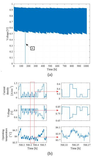
Figure 4.6 Cyclic dynamic loading for accelerated stress testing: (a) overall dynamic voltage; (b) around 500 hours, current density, voltage and operating temperature in one cycle, and zoom-in details.
