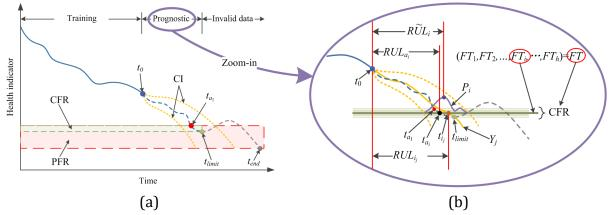
Figure 4.5 Schematic of hybrid prognostics: (a) segmentation of health indicator (data set), and failure ranges; (b) when prediction starting point is  $t_0$ , zoom-in prognostics part and predict remaining useful life.
