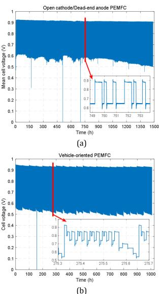
Figure 5.4 Voltage profiles of dynamic load cyclic from fuel cell ageing experiments, (a). FC-1; (b). FC-2.
