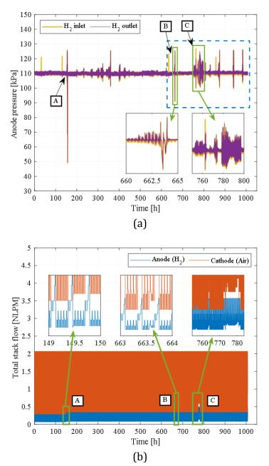
Figure 4.7 Anode gas pressure conditions and total stack flow, (a) the relationship between anode gas pressure and abnormal operation; (b) the relationship between total stack flow and abnormal operation.
