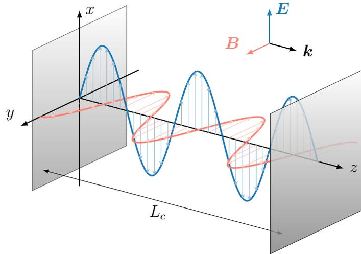
Figure 1.1: Schematic representation of an optical cavity consisting of two parallel mirrors separated by a distance of  $L_c$ , with electromagnetic fields propagating orthogonal to the mirrors, along the  $z$  direction. The mode function for an  $x$ -polarized electric field in the  $n = 5$  mode is sketched.
