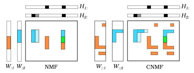
Figure 1. A visual comparison of NMF (left) and CNMF (right). CNMF allows to model complex time dependance while maintaining the number of templates low.
