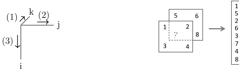
(a) Schematic representation of the order for unfolding/vectorizing, taken from [Coh15]. (b) Example of vectorization with a 2 \times 2 \times 2 tensor.
