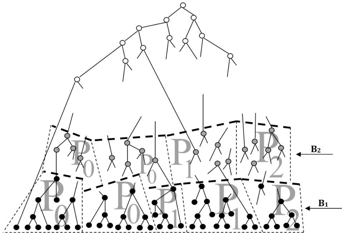
Figure 29 – Distribution scheme of blocks on three processors proposed by Kechid and Myoupo (2008b)
