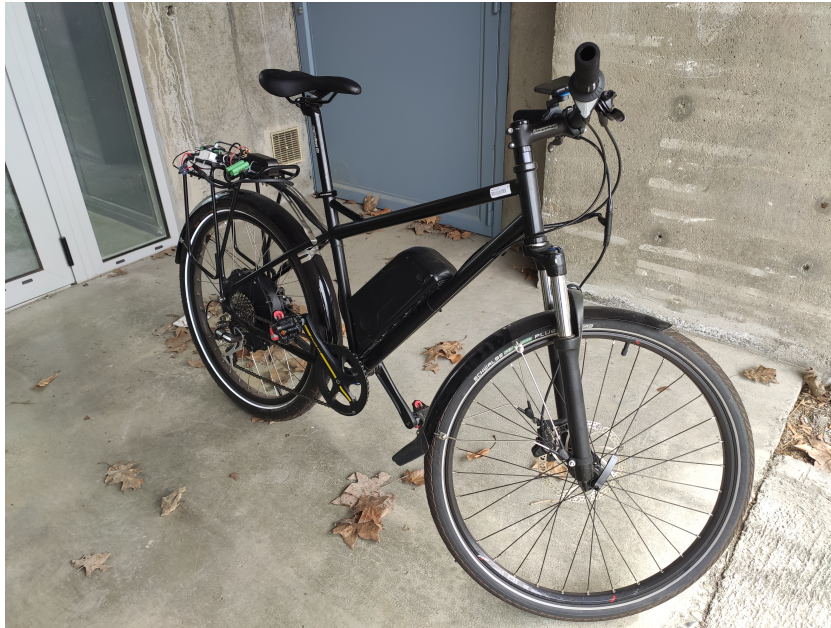
Figure 5.14: SPIRO E-bike prototype developed at Gipsa-lab.
