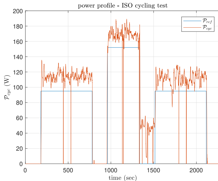
Figure 3.7: Power profile for the iso-power cycling test (ISO). The first and the last step are performed at 50% of the maximal power \mathcal{P}_{max} reached during the incremental cycling test (ICT) and the middle step is performed at 80% of \mathcal{P}_{max} .
