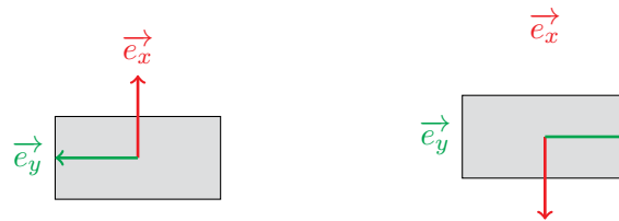
Figure 4.11 – Example of equivalent orientations for a rectangular cross-section.
