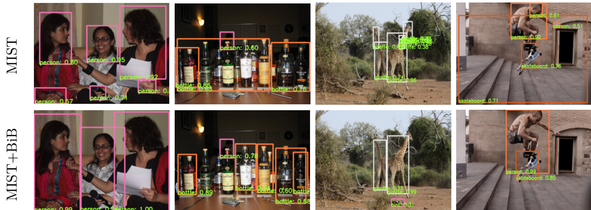
Figure 6.5 – Examples of predictions on the VOC07 and COCO test sets, by MIST [Ren, 2020a] (first row) and BiB after the first cycle (second row). Fine-tuning MIST with images selected by BiB significantly remedies its limitations.
