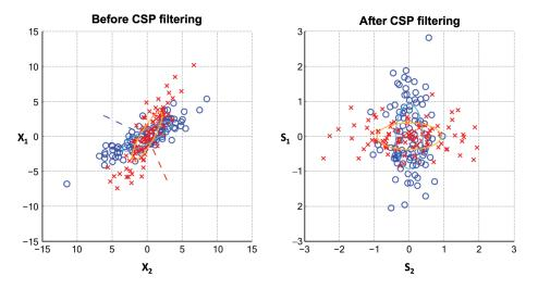
FIGURE 4.1: **CSP filtering**. On the left, the distribution of samples before filtering. Two ellipses show the estimated covariances and dashed lines show the direction of CSP projections. On the right, the distribution of samples after the filtering. The horizontal (vertical) axis gives the largest variance in the red (blue) class and the smallest in the blue (red) class, respectively. Extracted from Blankertz et al., 2007
