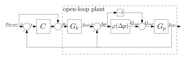
Figure 4.13: Block diagram of the full ventilation system, with  $G_b$  the blower dynamics, C an arbitrary feedback controller,  $G_p$  the patient-leak dynamics, and  $\varphi(\Delta p) = R_{hose}(\Delta p) + \ell \Delta p$  the nonlinear hose model.
