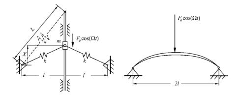
Figure 3.1: Mechanical structure of the elastic bar
