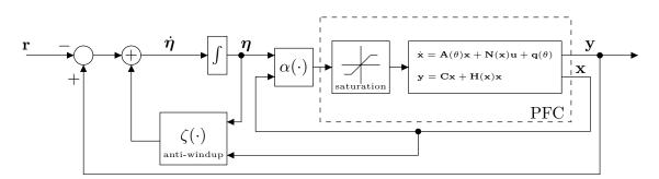
Figure 4.3: Proposed control structure for the PFC
