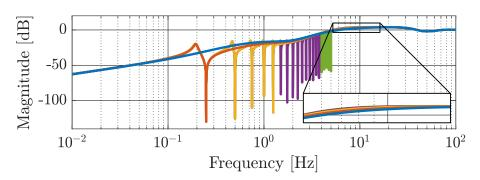
Figure 4.21: Bode magnitude plot of the sensitivity  $S_{re}$  for the linearization of the closedloop system with L = 0 (—), L = 1 (—), L = 5 (—), L = 15 (—), and L = 20 (—). The figure shows a magnitude increase at frequencies around 8 Hz, causing oscillations at these frequencies.
