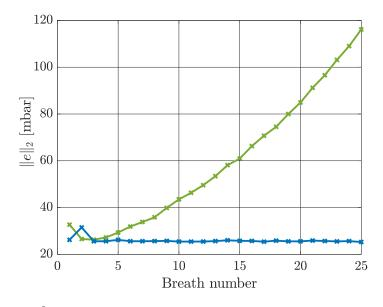
Figure 4.20: The  $\mathcal{L}^2$ -norm of the error for every breath for L = 0 (—), and L = 20 (—) for the baby use-case. The figure shows unstable behavior for that the closed-loop system with L = 20.
