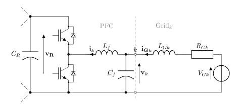
Figure 4.2: Detail of the k-th branch of the PFC (left) and the proposed Thevenin grid model as seen by this terminal (right)
