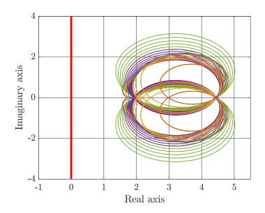
Figure 4.16: Nyquist plot of G(s) for L = 0 (—), L = 1 (—), L = 5 (—), L = 15 (—), and L = 20 (—). The figure shows that  $\operatorname{re}(G(j\omega)) > 0 \forall \omega \in [-\infty, \infty]$ .
