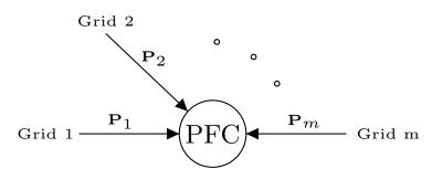
Figure 4.1: *m*-terminal PFC at a node in the grid
