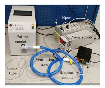
Figure 4.14: The experimental setup with the mechanic patient simulator, the respiratory module, ventilation hose, and dSPACE module.
