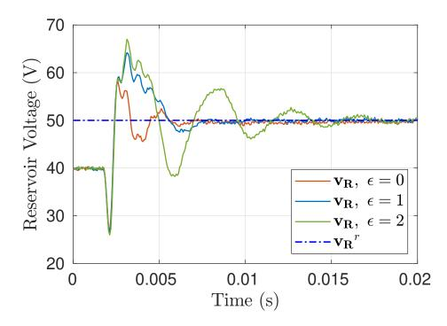
Figure 4.8: Experimental measurements of the startup of the converter on the nominal set-point for different values of  $\Omega = \epsilon I$ . Only  $\mathbf{v}_{\mathbf{R}}$  is shown, but the same behavior is observed on the other outputs
