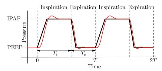
Figure 4.10: Typical airway pressure for two breathing cycles of pressure-controlled ventilation, showing the set-point (--) and the typical response (--).
