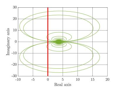
Figure 4.19: Nyquist plot of G(s) for L = 20 (----) for the baby use-case. The figure shows that  $\operatorname{re}(G(j\omega)) > 0 \forall \omega \in [-\infty, \infty]$  does not hold, hence, convergence is not guaranteed.
