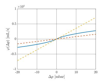
Figure 4.15: Visualization of the nonlinearity  $\varphi(\Delta p)$  (—), and its sector bounds  $\underline{\varphi}\Delta p$ (---) and  $\overline{\varphi}\Delta p$  (---), showing that the incremental sector condition holds for  $[\underline{\varphi}, \overline{\varphi}] = [80, \frac{1}{R_1} + \eta].$
