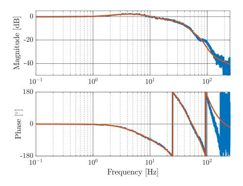
Figure 4.12: Frequency response measurement (-) and  $6^{\text{th}}$  order identified parametric model (-) of the blower, i.e., from  $p_c$  to  $p_{out}$ .
