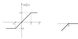
Figure 1: Function  $\operatorname{sat}_{s}^{\overline{s}}(s)$
