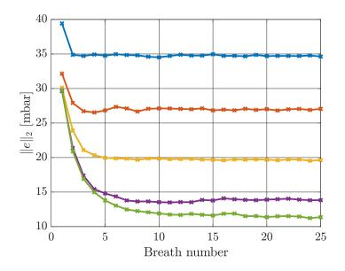
Figure 4.18: The  $\mathcal{L}^2$ -norm of the error for every breath for L = 0 (—), L = 1 (—), L = 5 (—), L = 15 (—), and L = 20 (—). The figure shows that more oscillators results in a smaller error and the controllers converge in approximately 10 breaths.
