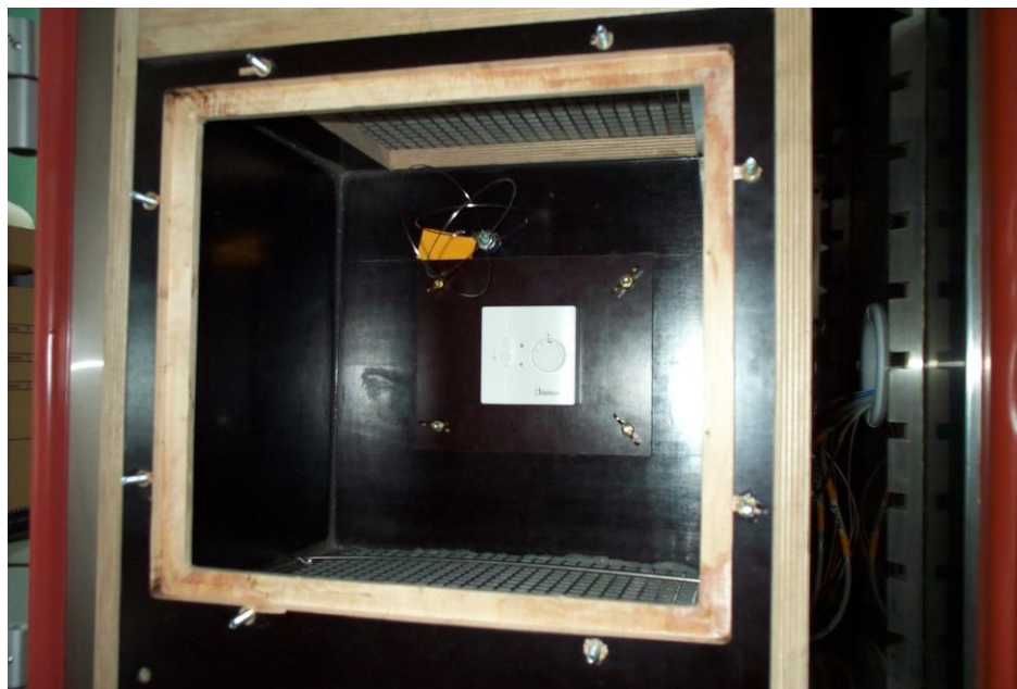
Figure 88: Air interface for controllers (inside view with controller)
