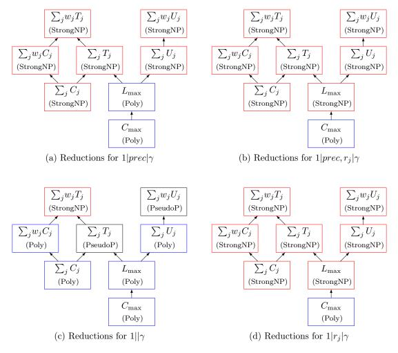
Figure 1.16: Reduction graphs and complexity classes of single-machine problems
