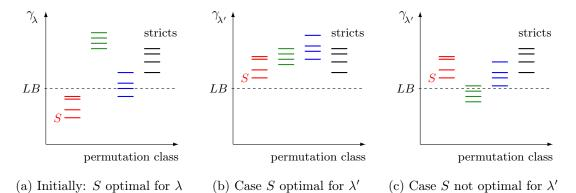
Figure 5.3: Refining a search for a dual Lagrangian optimum
