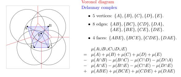
Figure 2.11: Surface of a union of disks using a Voronoï/Delaunay based abstract tube
