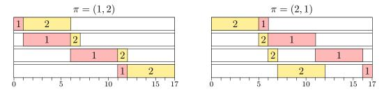
Figure 4.5: An instance of the  $F4|prmu|C_{max}$  problem and its two optimal solutions
