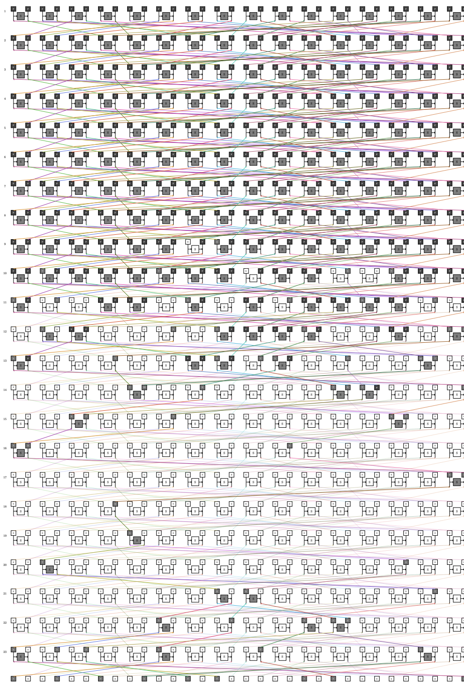
Figure B.2: Lower trail of the 23-round Boomerang distinguisher on WARP.
