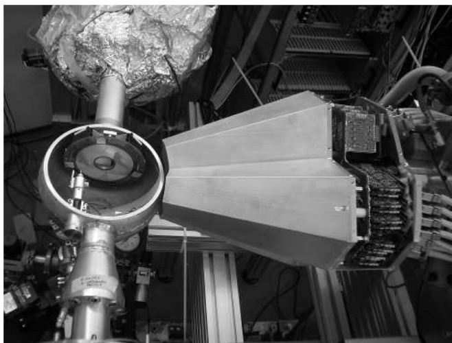
Figure 5.6: Photo of the experimental setup used to measure the position resolution of the AGATA triple cluster prototype. To the left inside the target chamber the double sided silicon strip detector is visible with the AGATA triple cluster in the center of the picture. Picture taken from Recchia et al. [244].
