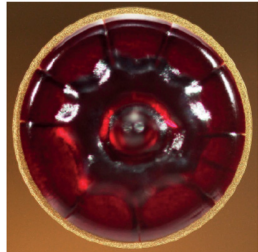
Fig. 9 Comparison with experiments by Pauchard and Allain [10] performed using a polymer drop; the two dried drops had almost the same contact angle and evaporated at the same room humidity. The initial diameter was also almost the same.
