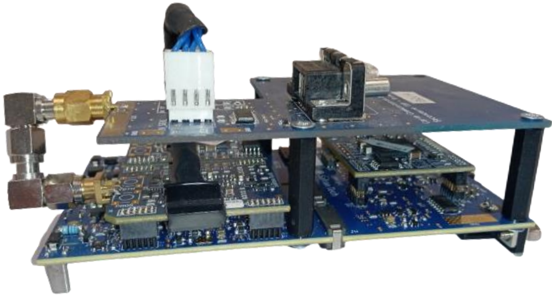
Figure 70. Ensemble gate-driver et carte de communication
