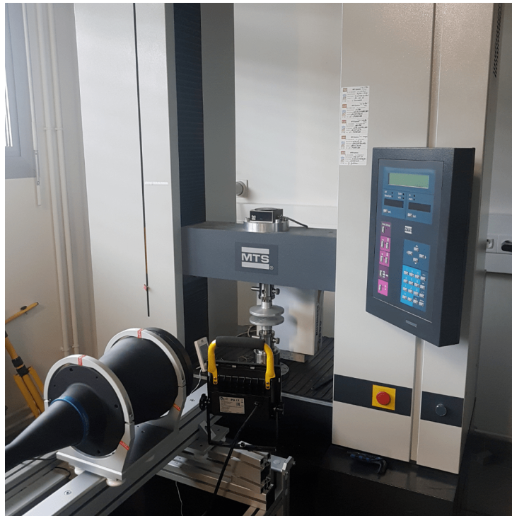
FIGURE 2.5 – Machine de traction (mode compression)
