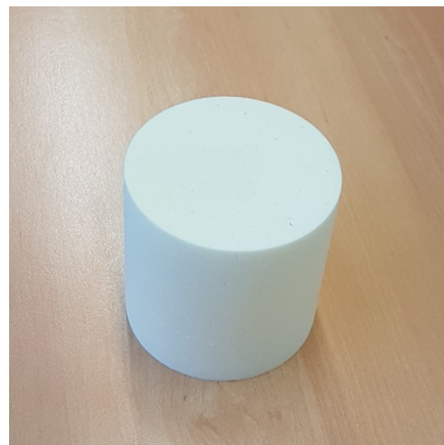
FIGURE 2.1 – Mousse de polyisocyanurate industrielle (Recticel) [26]
