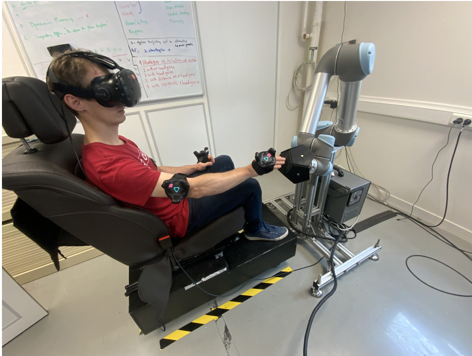
Figure 5.1 – The complete system setup for human-robot interaction.
