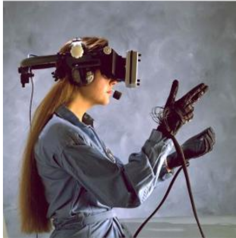
Figure 1.2 – Classic HMD and VR glove environment. [54]
