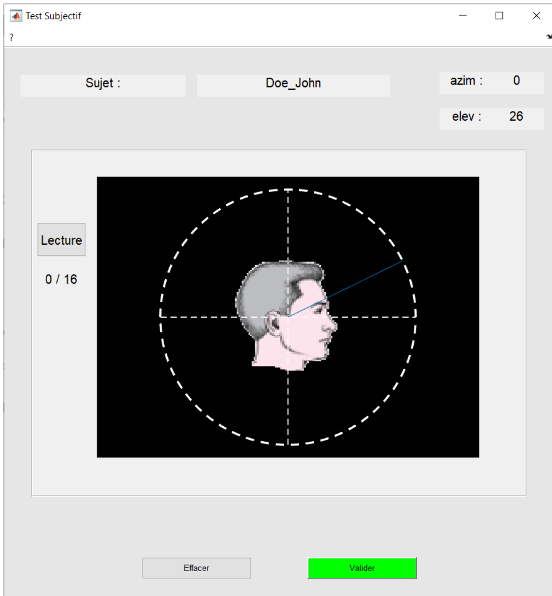
Figure 4.12 – Screenshot of the 2-D graphical user interface used to report the perceived direction of the stimuli in the median plane.
