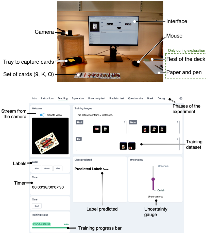
Figure 4.11. Top : The setup includes a screen, mouse, and camera stand for recording individual cards. Participants have access to the 12 training cards, the rest of the deck, paper and pens. Bottom : The application displays the live webcam feed, training set, prediction, uncertainty estimation and a series of tabs associated with each step of the experiment. The above interface is not shown in full screen for legibility. During the experiment, the different components are arranged in the same way but in full screen format.
