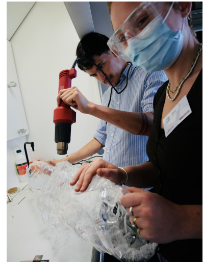
Figure 5.10: Manufacturing of the shell of Cor Epigloatte, with acrylic melted with a heat gun.
