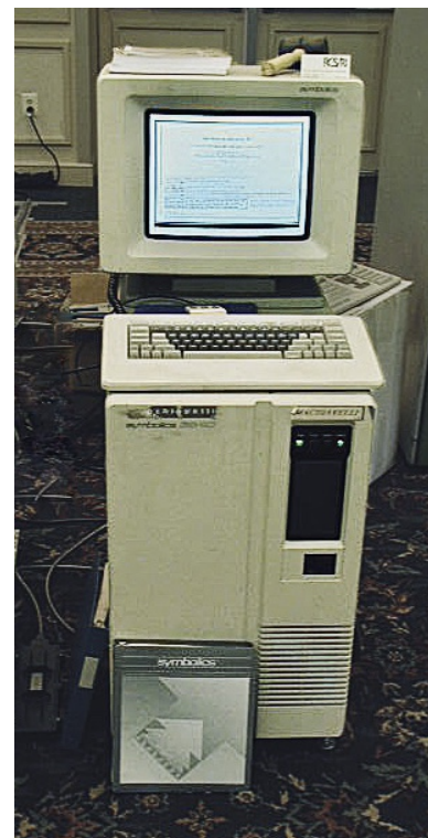
Figure 6.3: An example of LISP machine , vector of the expert systems diffusion in the 1980s. The model shown is a Symbolics 3640.
