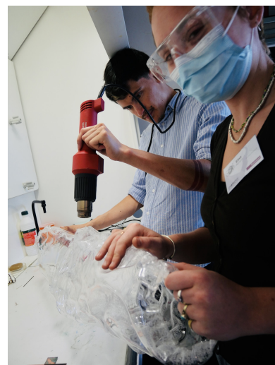
Figure 5.10: Manufacturing of the shell of Cor Epigloatte , with acrylic melted with a heat gun.
