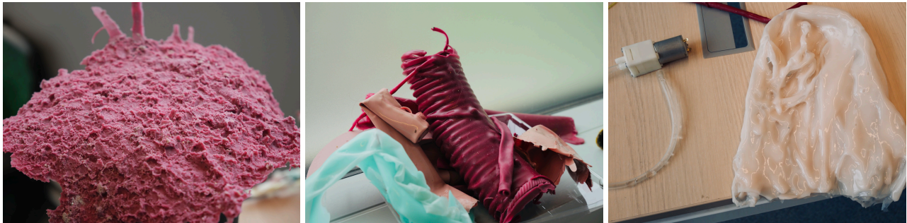
Figure 5.9. Organs artefacts obtained by molding silicone on different objects and surfaces.
