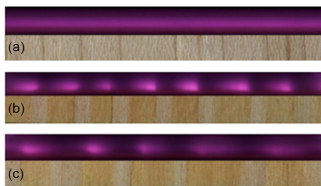
Figure 2. Spatial distribution of the helium plasma in presence of a sugar maple substrate (a) and Douglas pine samples with tight (b) and wide (c) late and early wood sections.
