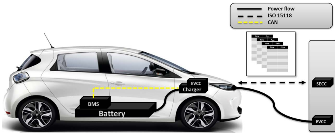
Figure 3.4 – Synoptic of EV charging
