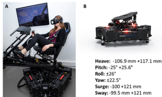
Figure 9.4 – Virtual reality motion platform (VRTigo, 6 dof) to be used for the ATARRI and TELECOG projects.
