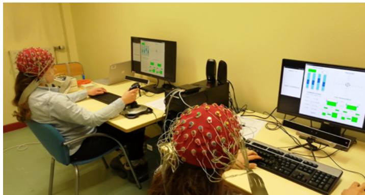
Figure 8.15 – From (Roy et al., 2020b): Hyperscanning setup with teammates equipped with a 64 electrode EEG system that perform an adapted Multi-Attribute Test Battery (MATB) task (pilot flying and pilot monitoring simulation).
