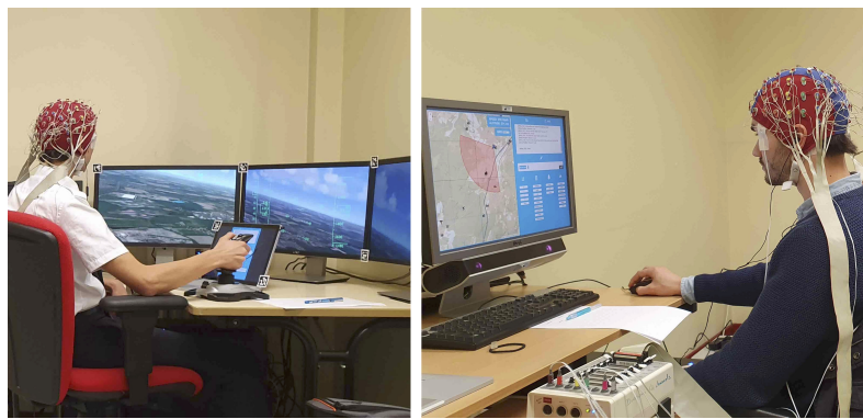
Figure 7.18 – From (Dehais et al., 2021): Hyperscan experimental setup: the Pilot (left) is flying the aircraft and exchanges instructions via a tablet with the JTAC (right) who is in charge of supervising the aircraft trajectory and gives instructions to the Pilot via the user interface.
