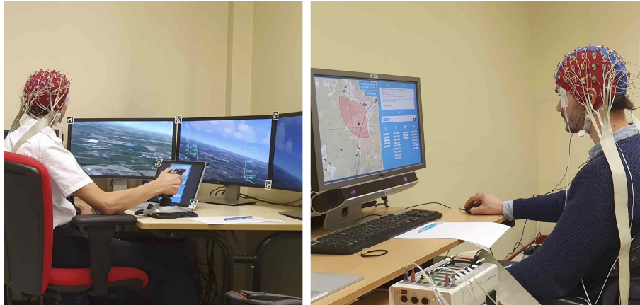
Figure 8.18 – From (Dehais et al., 2021): Experimental setup: the Pilot (left) is flying the aircraft and exchanges instructions via a tablet with the JTAC (right) who is in charge of supervising the aircraft trajectory and gives instructions to the Pilot via the user interface.
