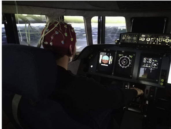
Figure 8.7 – From (Dehais et al., 2019c): ISAE-SUPAERO three axis motion flight simulator. The participants were left seated and equipped with a Biosemi 32-electrode EEG system.
