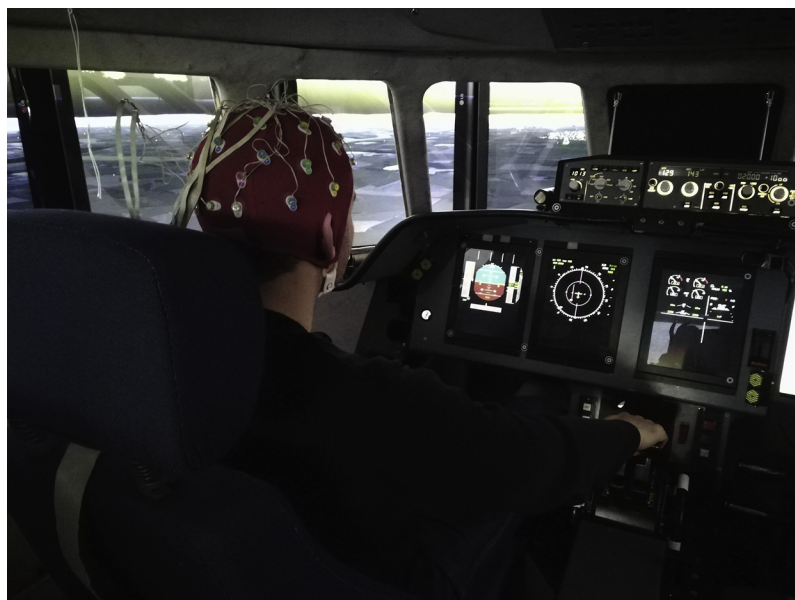
Fig. 3. ISAE-SUPAERO three axis motion flight simulator. The participants were left seated and equipped with a Biosemi 32-electrode EEG system.
