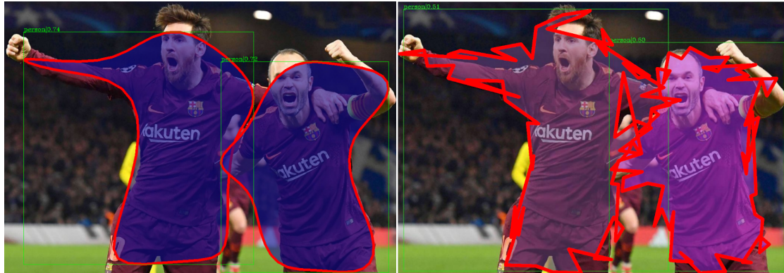
Figure 4.12: Thanks to our coefficient regularization, our method ( left ) learns to regress smooth shapes, whereas the cartesian version of [MBZ20] ( right ) regresses erratic shapes when using a high number of coefficients (here 32).
