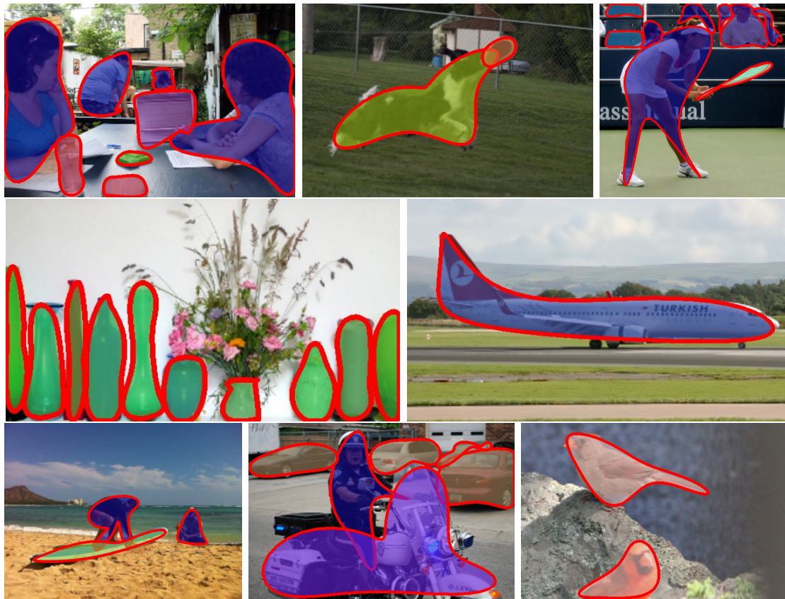
Figure 4.7: Our Smooth Contour Regression (SCR) algorithm captures the silhouette of objects with a compact resolution-independent representation based on Fourier coefficients. Contours produced by our algorithm adequately approximate the general shape of free-form objects such as persons, animals, cars, or pots while being defined in a simple parametric way with only a few complex Fourier coefficients, here 8. Images from COCO 2017 test-dev.
