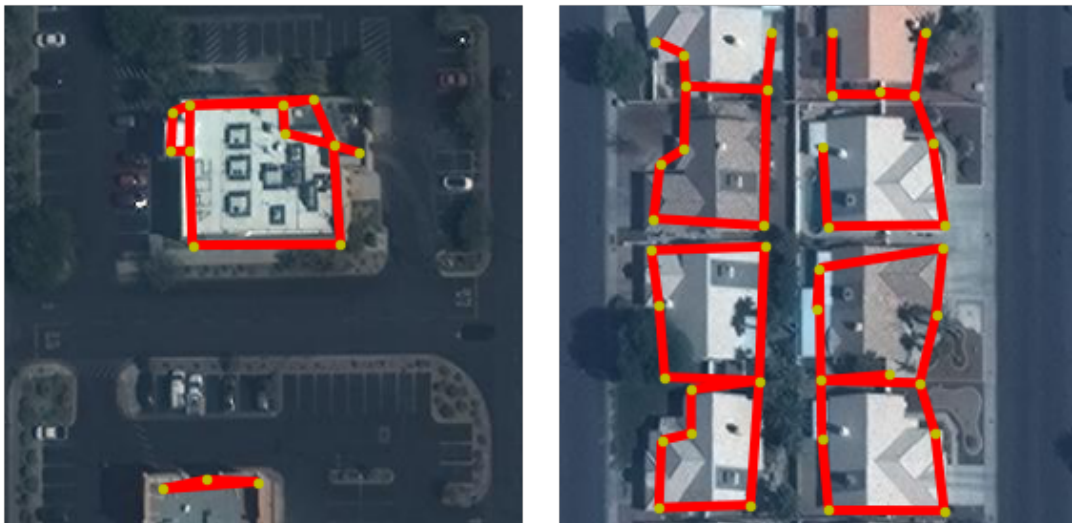
Figure 5.11: Our method can be used for other tasks, such as building extraction. This example is taken from the CrowdAI Mapping Challenge dataset [Moh+20]
