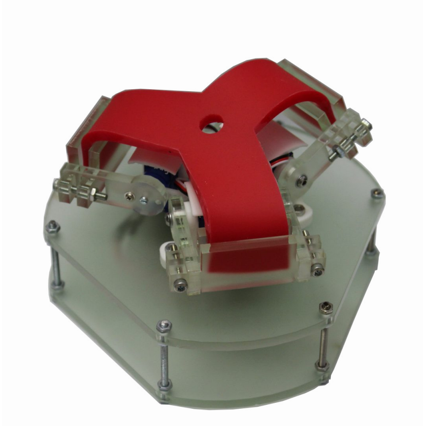
Figure 4.2: The Tripod Robot is composed of a soft silicone piece actuated by three servomotors, the robot can achieve a nearly infinite number of shape configurations.
