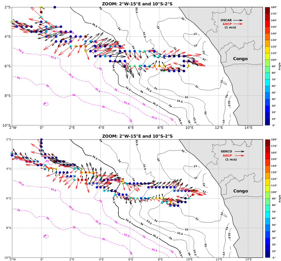
FIGURE 3.18 – Angular deviation between ADCP currents averaged over the depth of 30-m (from PIRATA FR27) and OSCAR (top panel) and GEKCO (bottom panel) products. Arrows are currents directions : black for OSCAR and GEKCO and red for ADCP currents. Colourous dots represent the associated angular values. SSS contours are shown : black contours for freshwater plumes and magenta contours for outside of plumes.
