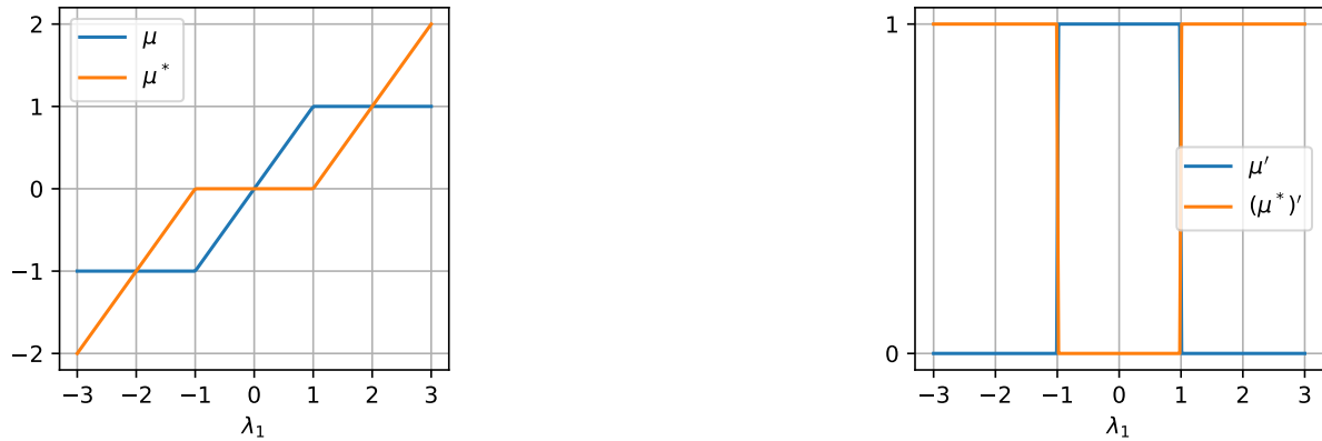
Figure 7.19 – (FDA) Dual functions \mu, \mu^* (left) and their derivative (right) used to implicitly parametrise the FDA relation (7.53). Note that similar functions have already been used (without being formalised) in figure 7.12 for the OPA.
