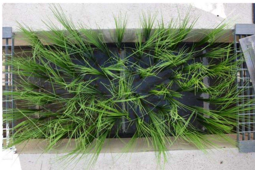
FIGURE 3 Picture of the vegetated area ( Isolepis sp.) in the experimental channel (36 plants per concrete panel on two panels)
