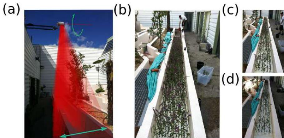
**FIGURE 1** Illustration of the experimental setup. (a) The laser scanner and its scanning view (in red) through the channel flume. (b), (c), and (d) An example of species planting (*Lythrum salicaria*) at densities of 41, 82, and 164 plants/m<sup>2</sup>, respectively
