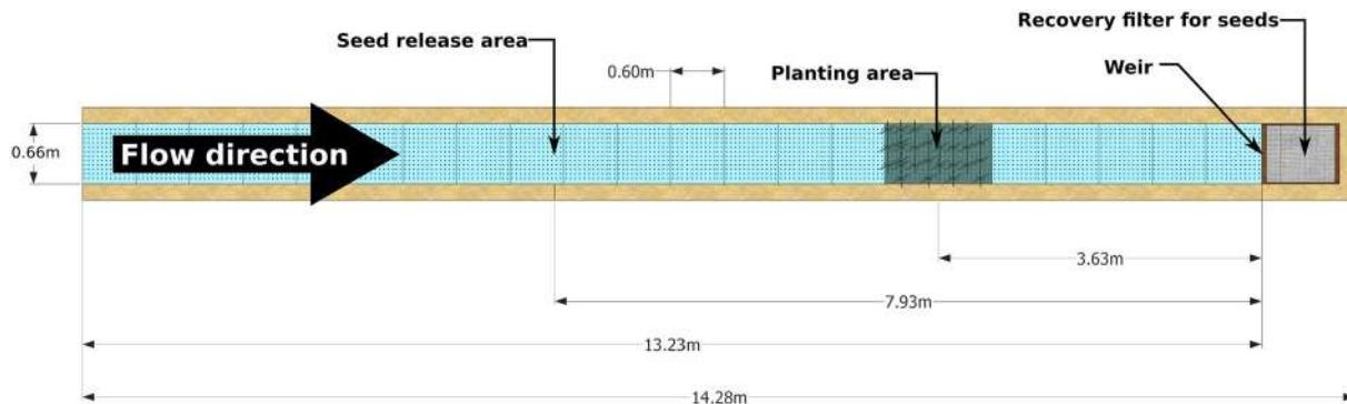
**FIGURE 1** Schematic representation of the experimental channel
