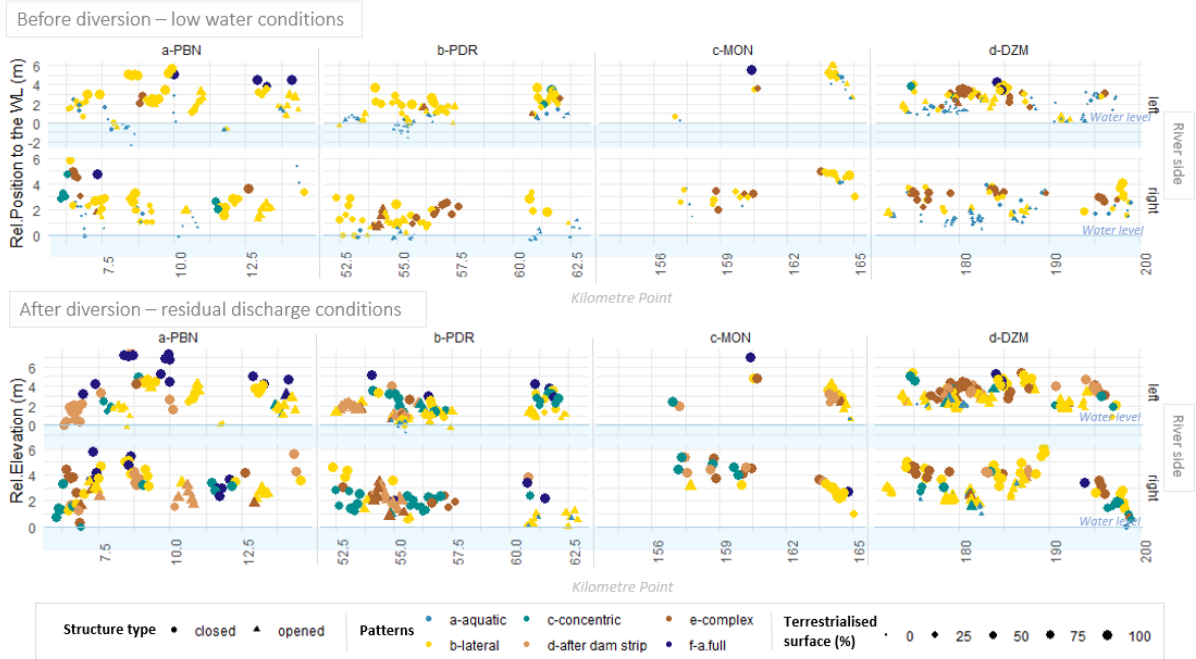
Figure 86 : Mean relative elevation of the dike structures to the water level at low flow, terrestrialized surfaces percentages and pattern zonation according to an upstream-downstream gradient in pre- and post-diversion conditions
