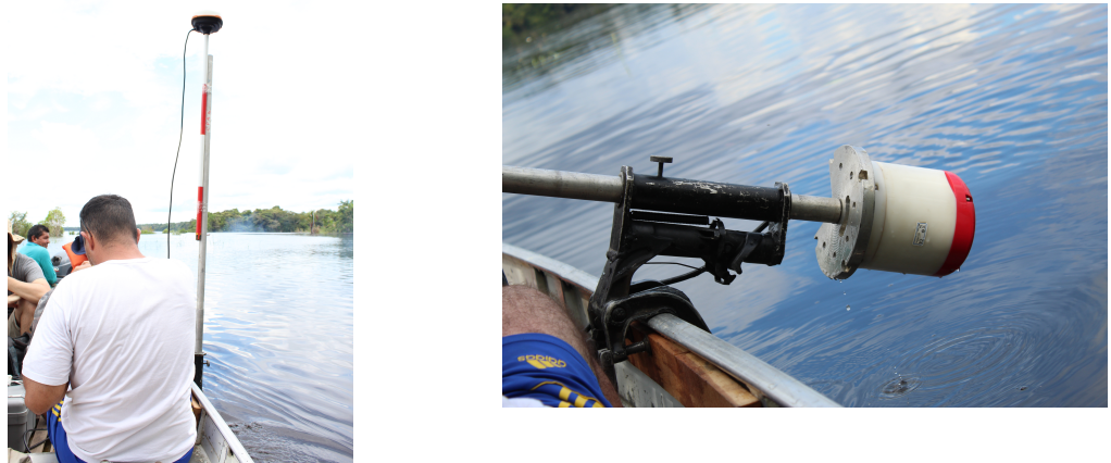
Figure 1.6: ADCP sensors mounted on a small boat (photograph by author, 2018). The top part of the metal bar is fitted with a GPS to track the boat position during a transect.
