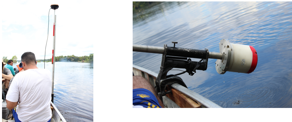
Figure 1.6: ADCP sensors mounted on a small boat (photograph by author, 2018). The top part of the metal bar is fitted with a GPS to track the boat position during a transect.
