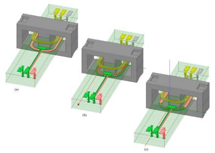
Figure IV-13: Renovated shielding structures (a) thin typical; (b) chopped; (c) asymmetrical
