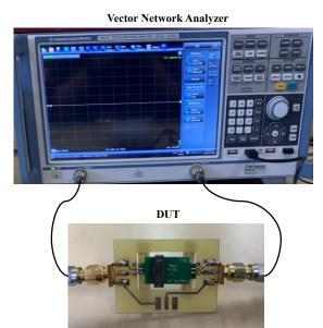
Figure III-19: S parameter experimental analysis using VNA
