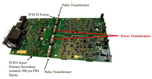
Figure III-8: Pulse transformers integrated in realized gate driver card [78]
