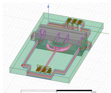
Figure II-7: Planar transformer ODB++ file imported directly into Q3D
