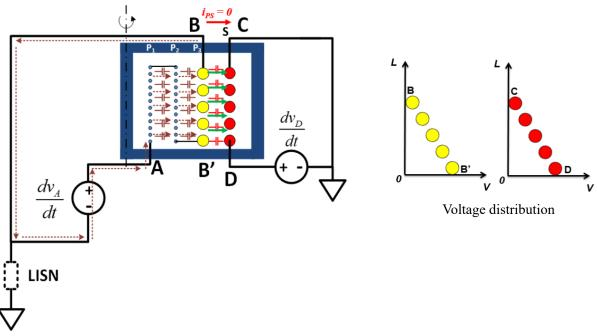
Figure I-29: Series shielding method [138]
