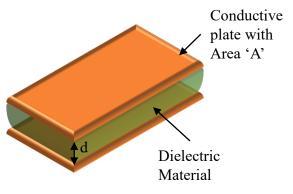
Figure II-4: Representation of a parallel plate capacitor
