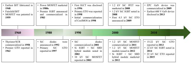
Figure I-7: Pivotal power semiconductor development and commercialization story line
