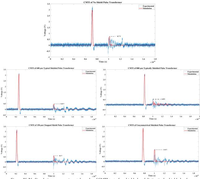
Figure IV-26: Simulation vs. experimental results of CMTI test of unshielded and distinctively shielded pulse transformers
