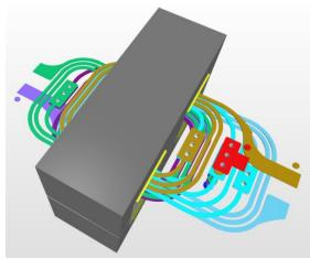
Figure II-6: Planar transformer design using Altium Designer
