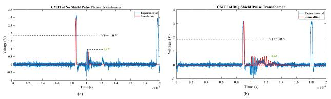
Figure III-29: CMTI test of pulse transformers (a) No shield; (b) Large shield
