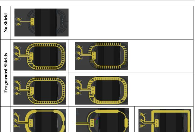
Figure IV-9: No shield, fragmented and solid shielding designs modelled in Altium Designer
