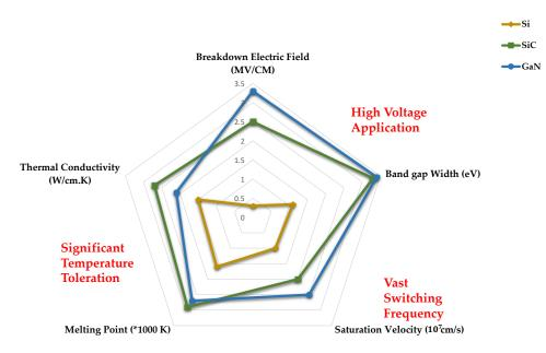
Figure I-8: Intrinsic properties of semiconductor materials: Si, SiC, GaN
