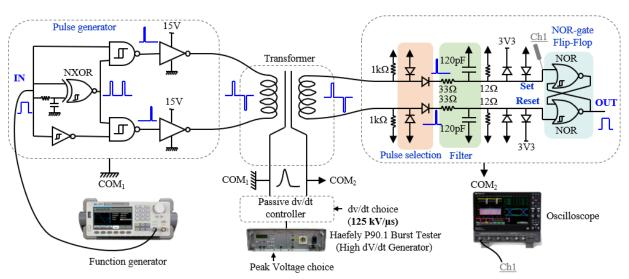
Figure IV-23: Pulse transformer susceptibility test circuitry to an application of 125 kV/µs between its disparate grounds
