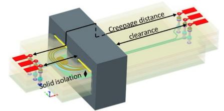
Figure IV-3: Pulse transformer configuration in compliance to electrical isolation standards
