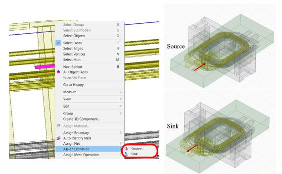
Figure II-17: Assigning excitations on planar transformer nets
