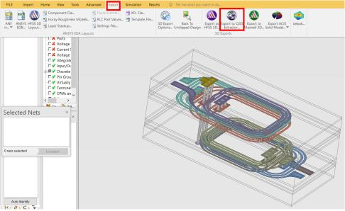
Figure II-14: Export to Q3D Extractor from Ansys SIWAVE
