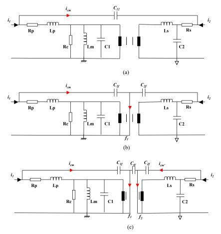
Figure III-3: CM model of a planar transformer (a) without shielding; (b) with one shield; (c) with two shielding layers
