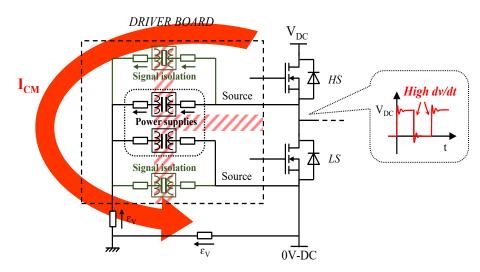
Figure I-23: Common mode current modelling through galvanic isolation of gate driver boards[78]
