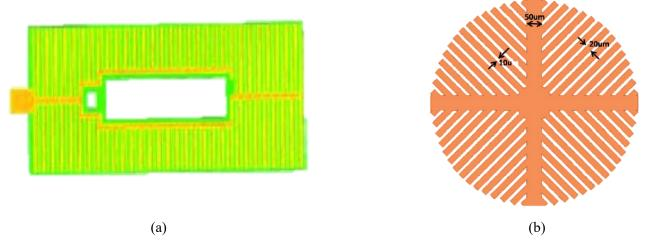
Figure I-32: Novel faraday shield (a) comb-shaped [136]; (b) patterned [135]
