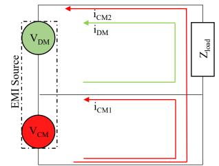
Figure I-22: Conducted DM and CM propagation in an electrical circuit
