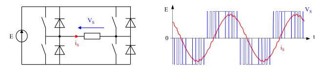
Figure I-5 : Single-phase full bridge inverter with associated waveforms
