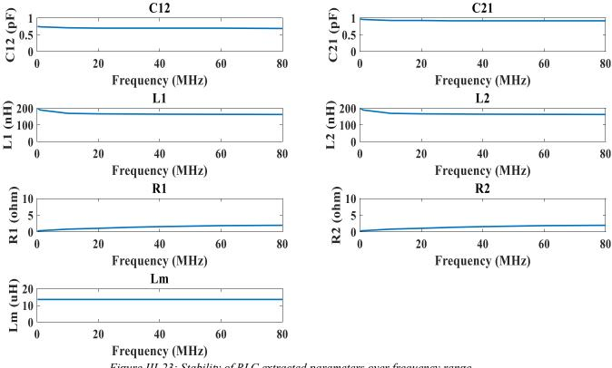
Figure III-23: Stability of RLC extracted parameters over frequency range
