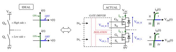
Figure I-6: Basic example of a switching arm with N-MOSFET transistors
