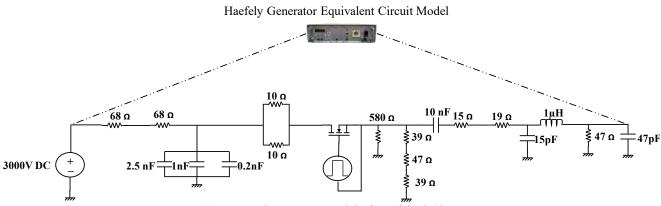
Figure IV-22: Equivalent circuit model of Haefely dv/dt generator
