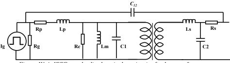
Figure IV-4: IEEE standardized equivalent circuit of pulse transformer
