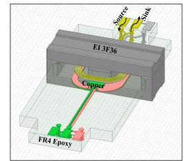
Figure III-17: Pulse transformer setup in Ansys Q3D Extractor
