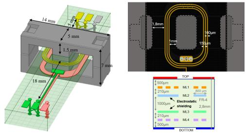
Figure IV-5: Pulse planar transformer synopsis
