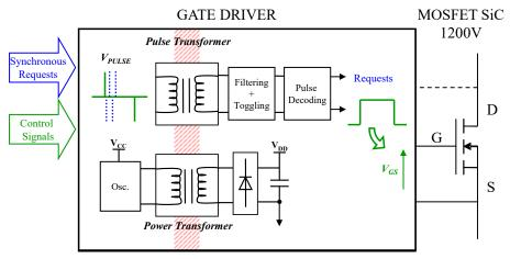
Figure III-10: Principle of operation of data signal transmission
