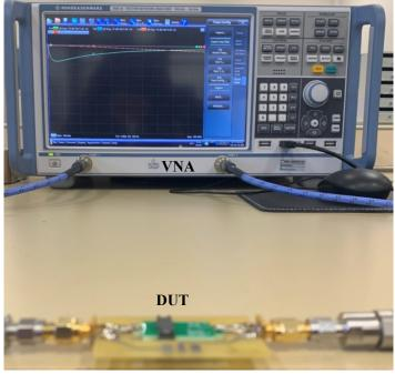
Figure IV-14: Experimental S parameter analysis
