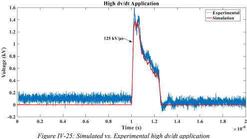
Figure 17-25. Simulated VS. Experimental high dv/al application
