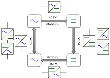
Figure I-2: Basic forms of power converters
