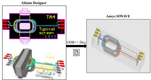
Figure III-14: Importing ODB++ files of Altium designed model into Ansys SIWAVE
