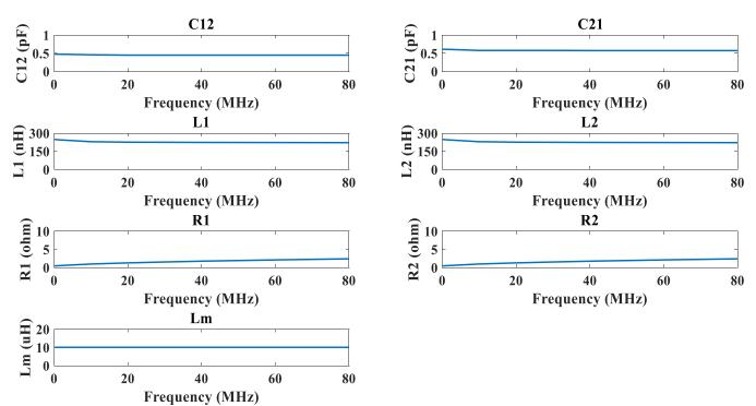
Figure IV-19: Steadiness of RLC extracted parameters over frequency bandwidth
