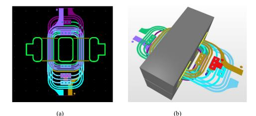
Figure II-10: Altium Designer power transformer model (a) 2-D representation; (b) 3-D representation
