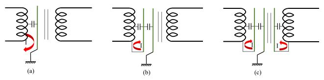
Figure I-28: Shielded isolation transformers (a) single-shield; (b) double-shield; (c) triple-shield
