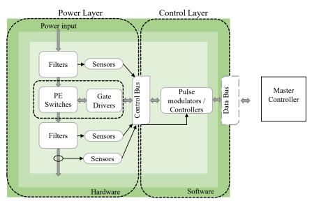
Figure I-4: Block diagram of power electronics arrangement
