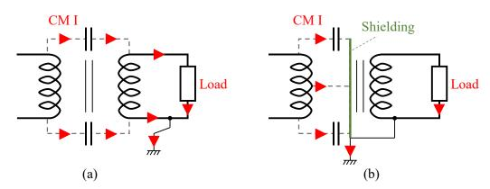
Figure I-27: CM current path in transformer (a) without shielding; (b) with grounded electrostatic shield
