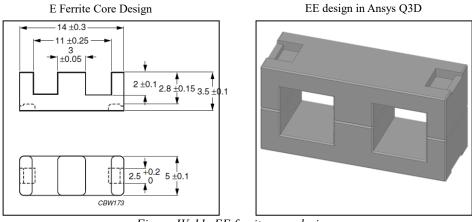
Figure IV-11: EE ferrite core design
