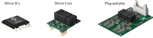
Figure I-12: Basic classes of gate drivers<sup>2</sup>
