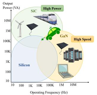
Figure I-9: Applications of SiC and GaN relative to operating frequency and output power
