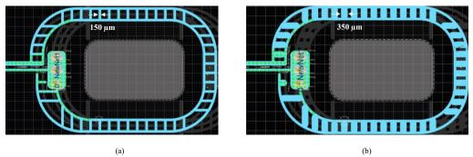
Figure IV-21: Fragmented shield structure of pulse transformer (a) 150 µm dissections; (b) 350 µm dissections
