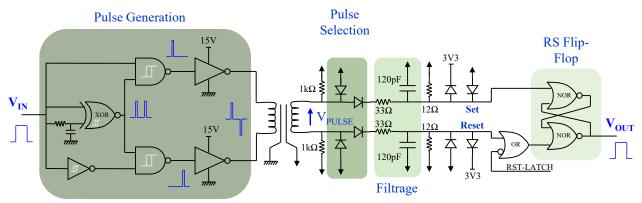
Figure III-12: Pulse transformer electronic circuitry
