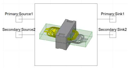
Figure II-24: Four-port subcircuit in Ansys Circuit Design
