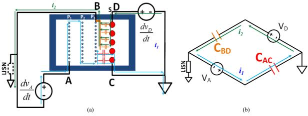
Figure I-30: Partial shielding method (a) configuration; (b) CM noise model [138]
