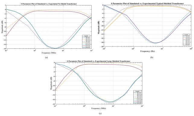
*Figure III-20: Experimental authentication of S parameter results of pulse transformers (a) No shield; (b) Typical shield; (c) Large shield*
