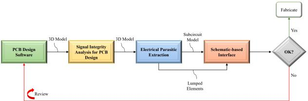
Figure II-8: Mechanism followed to simulate pulse transformer model
