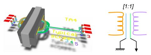
Figure III-6: Pulse planar transformer synopsis
