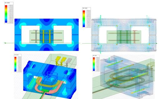
Figure IV-16: Magnetic field strength (magnitude and vector) demonstrated on the EE core of the typically shielded pulse transformer
