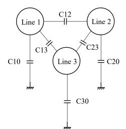
Figure II-3: Example of parasitic capacitance computation between three conductors
