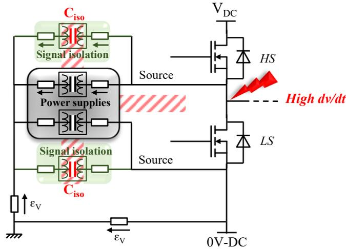
Figure III-2: Pulse transformer parasitic capacitances in a gate driver board
