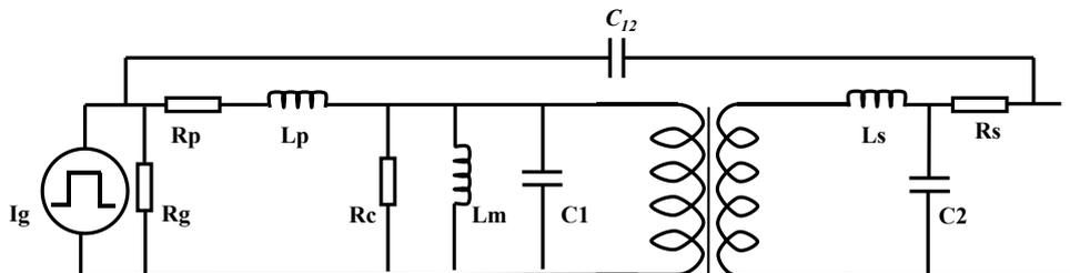
Figure IV-4: IEEE standardized equivalent circuit of pulse transformer
