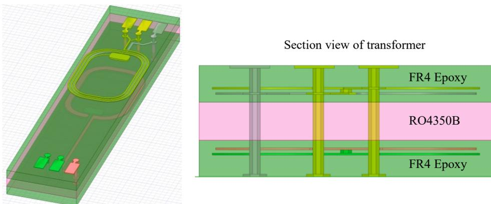
Figure IV-27: Hybrid dielectric material assignment in Ansys Q3D
