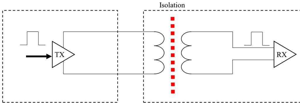
Figure I-14: Composition of an integrated inductive isolator
