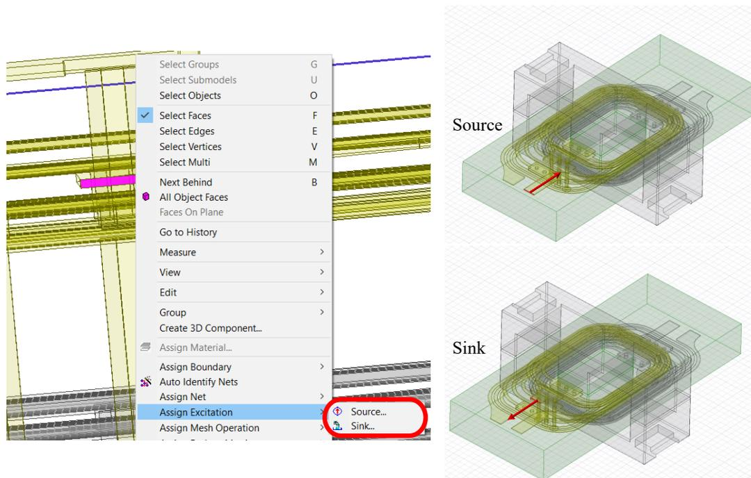
*Figure II-17: Assigning excitations on planar transformer nets*
