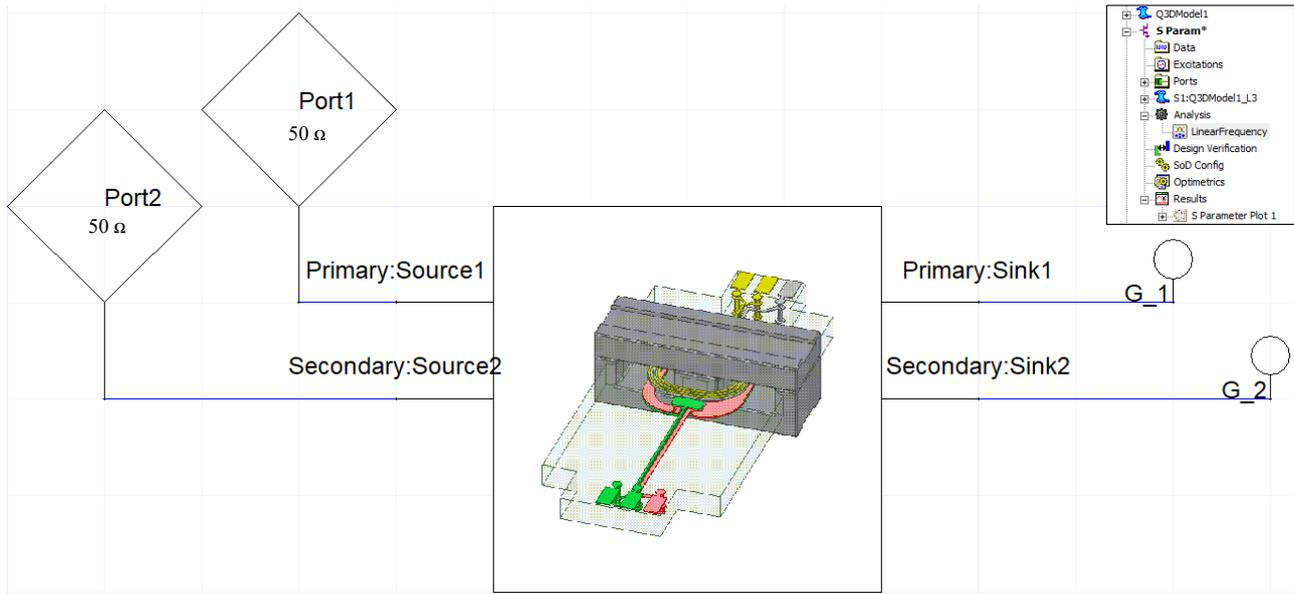
Figure III-18: S Parameter simulation analysis of dynamically linked model in Ansys Circuit Design
