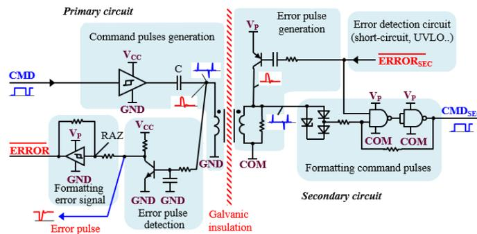
Figure III-5: Error pulse circuit configuration utilizing pulse transformer
