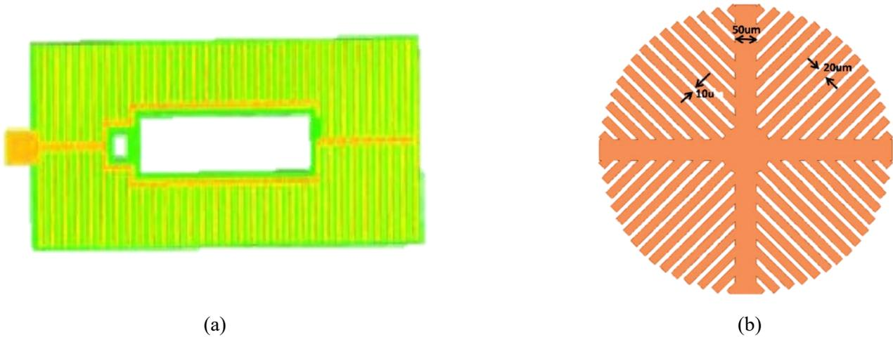
Figure I-32: Novel faraday shield (a) comb-shaped [136]; (b) patterned [135]
