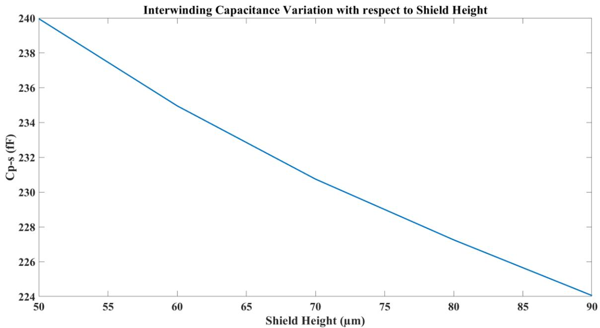
Figure IV-8: Interwinding capacitance variation according to shield height
