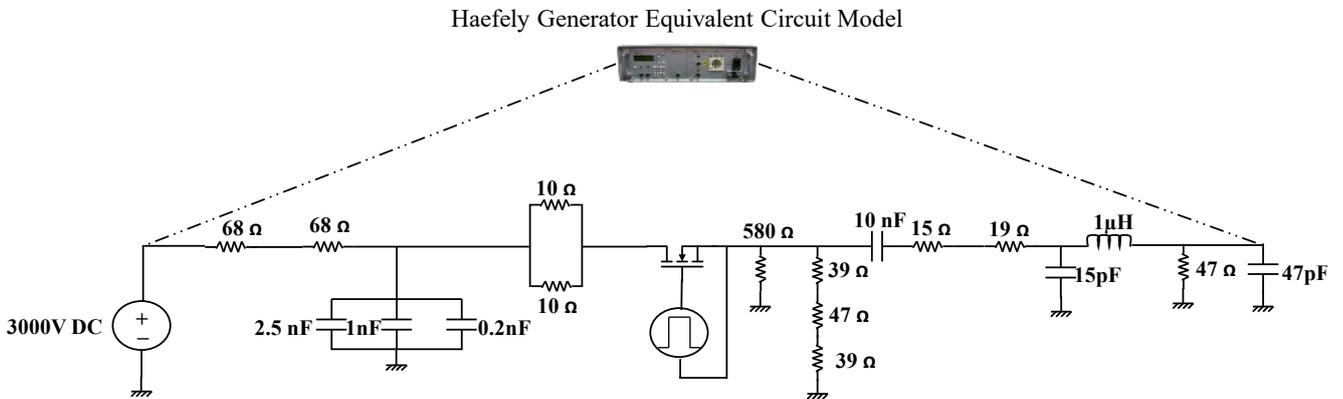
Figure IV-22: Equivalent circuit model of Haefely  $dv/dt$  generator
