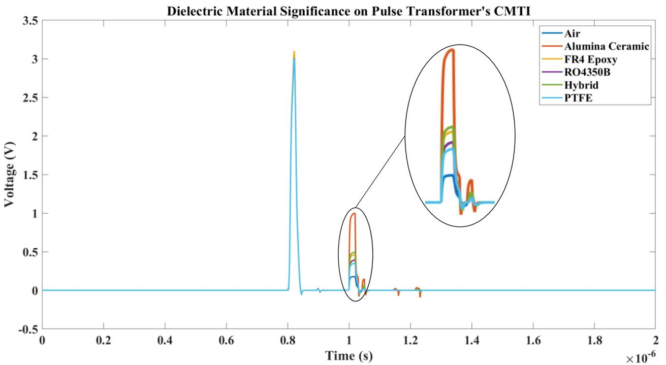
Figure IV-28: Dielectric material effect on transformer's CMTI
