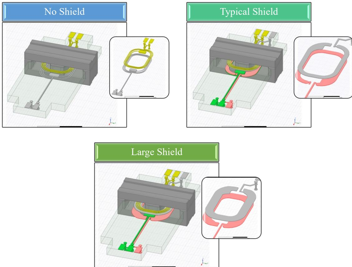
Figure III-16: No shield, typical shield and large shield pulse transformers in Ansys Q3D
