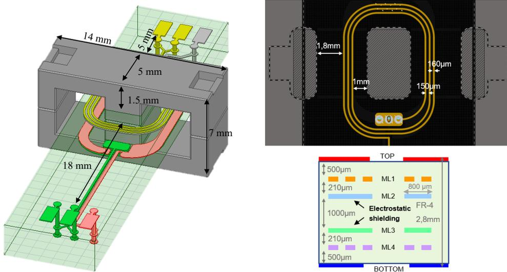
Figure IV-5: Pulse planar transformer synopsis
