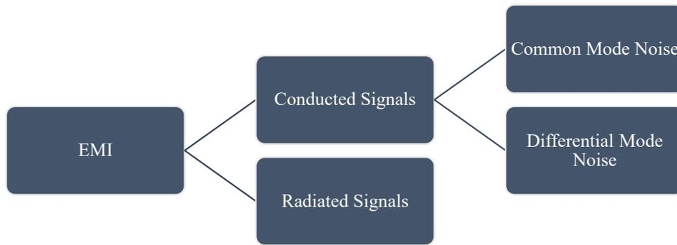
Figure I-21: Classification of EMI signals in electrical circuits
