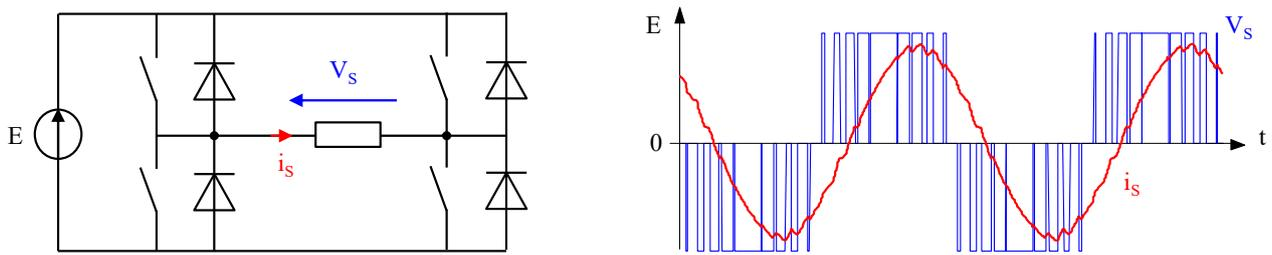
Figure I-5 : Single-phase full bridge inverter with associated waveforms
