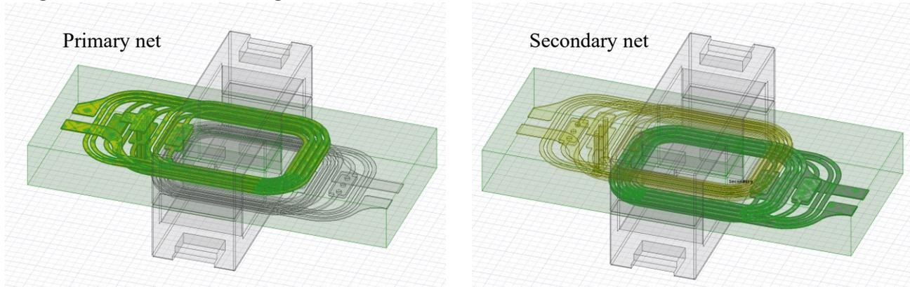
Figure II-16: Assigning the transformer nets in Ansys Q3D
