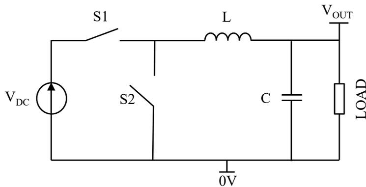
Figure I-3: Ideal DC-DC step-down converter circuit (buck converter)
