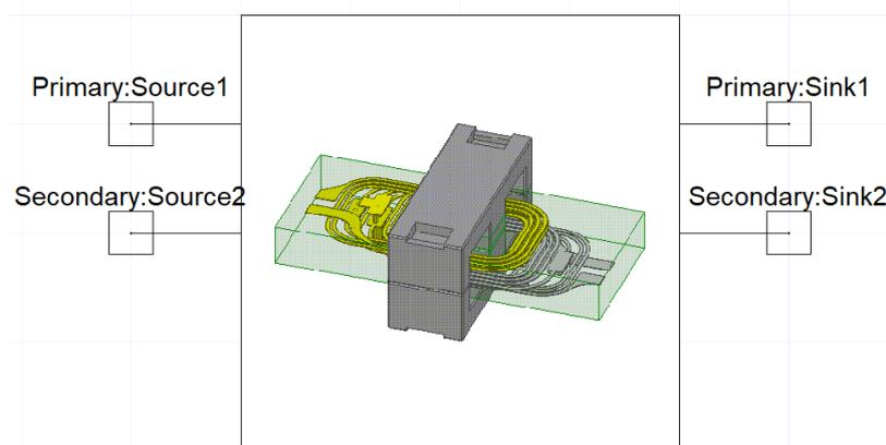
Figure II-24: Four-port subcircuit in Ansys Circuit Design
