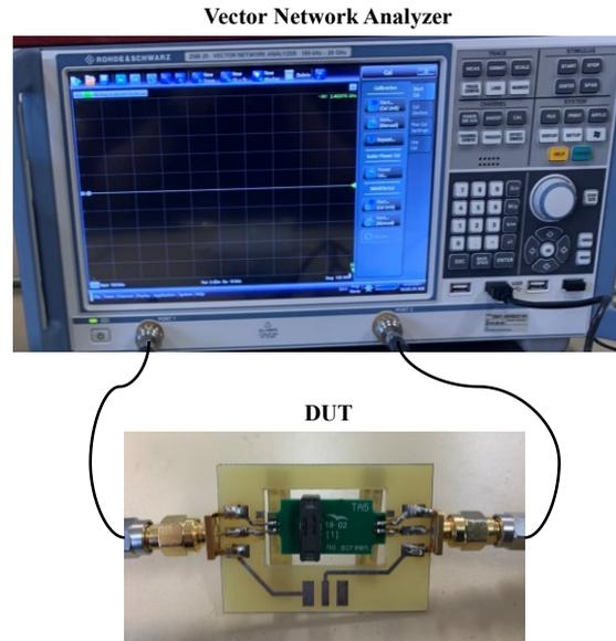
Figure III-19: S parameter experimental analysis using VNA
