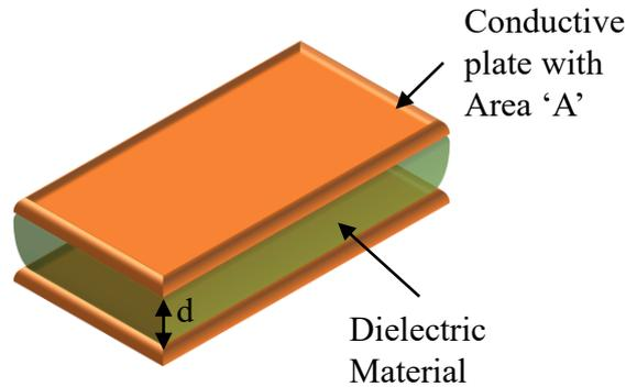
Figure II-4: Representation of a parallel plate capacitor
