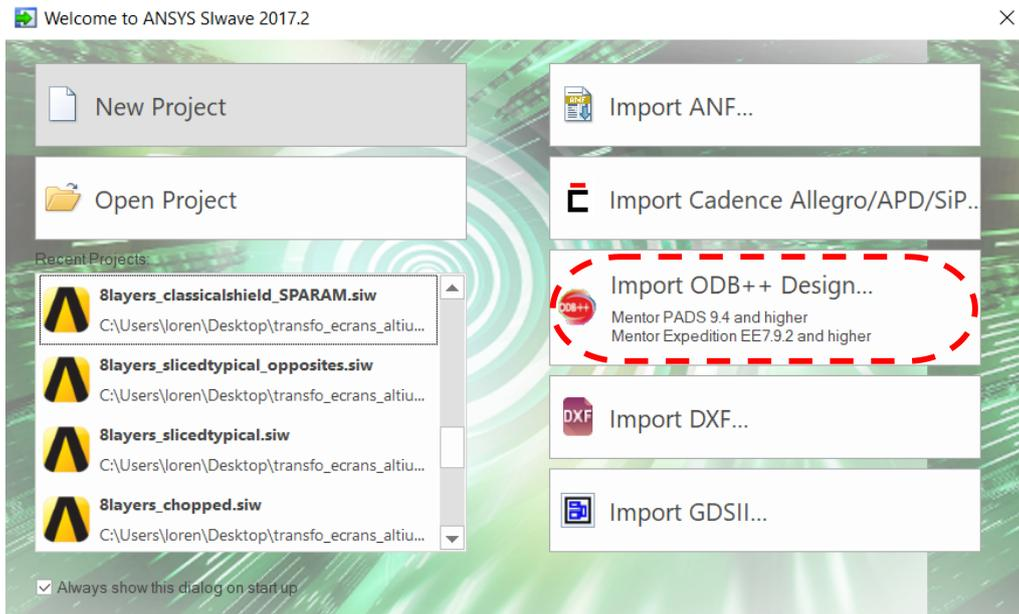
Figure II-12: Importing ODB++ files into Ansys SIWAVE
