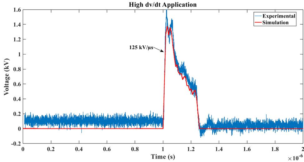
Figure III-27: Experimented vs. simulated abrupt dv/dt application
