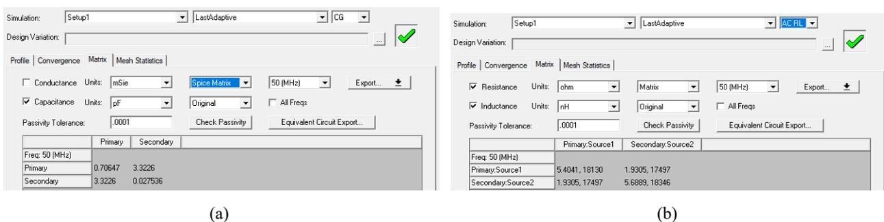
Figure II-22: Matrix solution data (a) capacitance matrix ; (b) AC RL matrix
