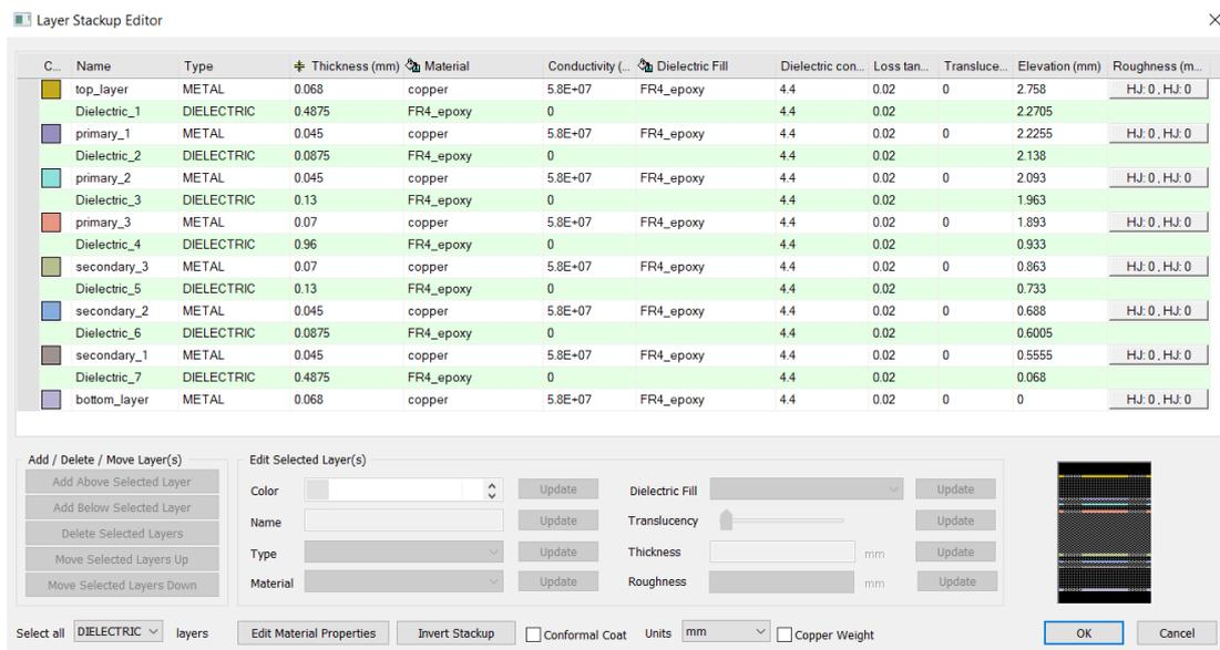
Figure II-13: Transformer layer stack-up editor in Ansys SIWAVE
