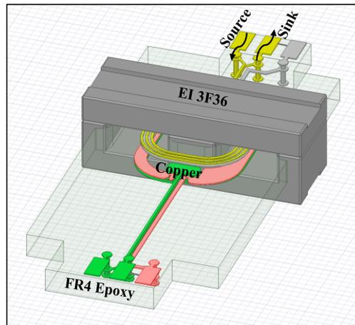
Figure III-17: Pulse transformer setup in Ansys Q3D Extractor
