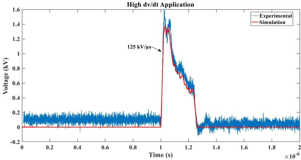
Figure IV-25: Simulated vs. Experimental high  $dv/dt$  application
