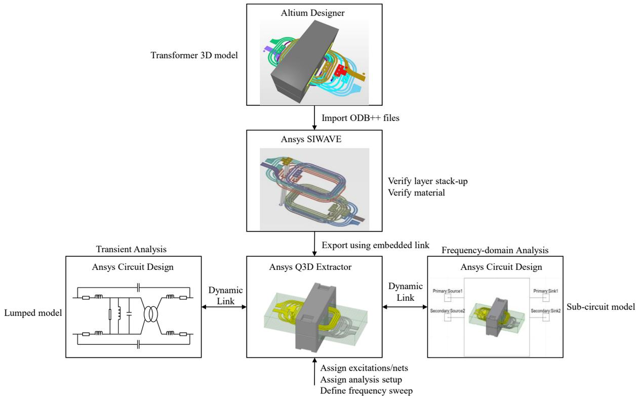
Figure II-9: Generic software scheme used to simulate planar transformers
