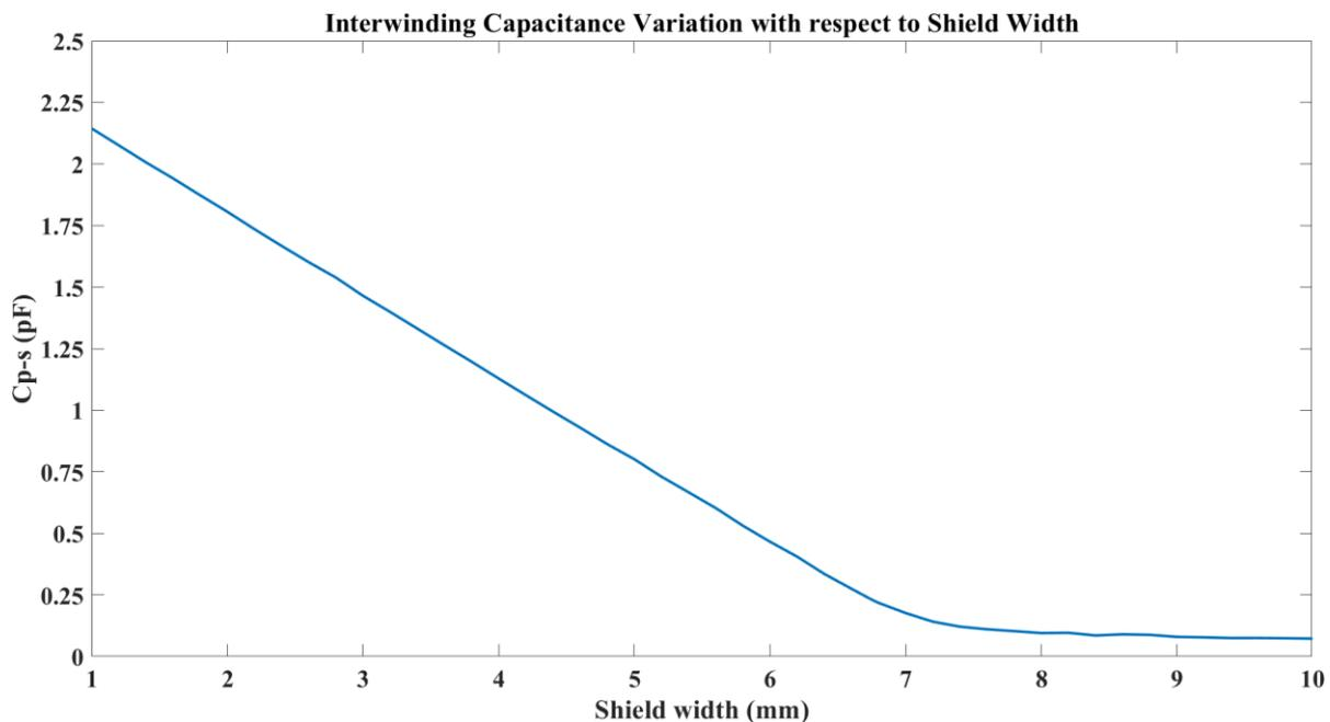
Figure IV-6: Interwinding capacitance variation according to shield width
