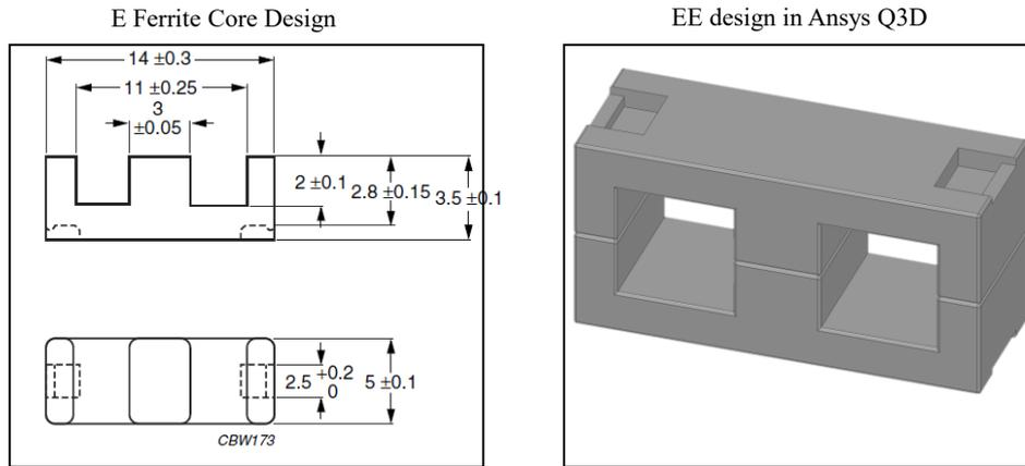
Figure IV-11: EE ferrite core design
