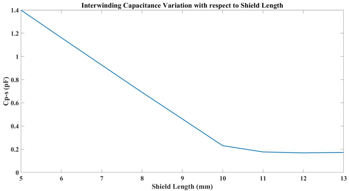
Figure IV-7: Interwinding capacitance variation according to shield length
