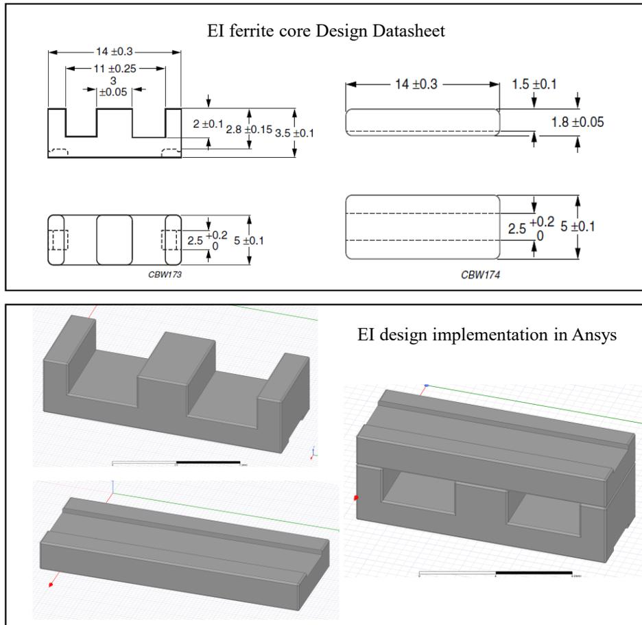
Figure III-15: EI ferrite core design specifications [223]
