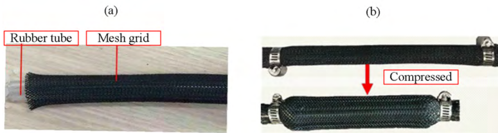
Fig. 2. 1: Mechanical design of McKibben Artificial Muscles: (a) basic components of the muscle (Zhao et al., 2018); (b) state of the muscle before and after compression (Zhao et al., 2017);
