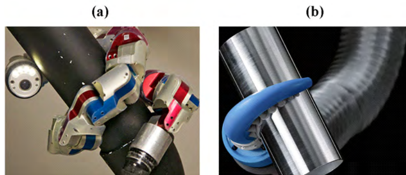
Fig. 1. 2: Examples of soft compliant robot end-effectors: (a) Snake Robots (Wright et al., 2012); (b): Soft Tentacle Gripper of Festo Company (Müller et al., 2020);
