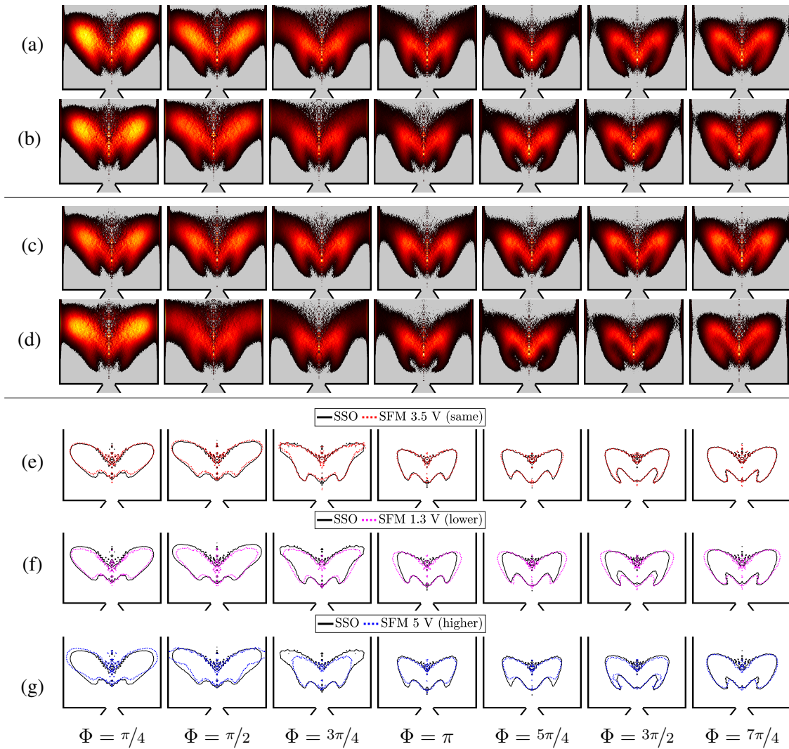
Figure 3.2. (a-d) Phase-averaged, Abel-inverted flame images shown in false colors. Light intensity of \text{OH}^* chemiluminescence is obtained at different phase instants of the acoustic cycle using an intensified camera. (a) Images obtained under SSO at a frequency f_0 = 533 Hz. I'_{\text{OH}^*}/\overline{I_{\text{OH}^*}} = 28.9\% . (b-d) Images corresponding to SFM at the frequency of SSO. (b) The forcing amplitude matches that observed during SSO ( I'_{\text{OH}^*}/\overline{I_{\text{OH}^*}} = 30.4\% ). (c) The forcing amplitude is lower than that observed during SSO ( I'_{\text{OH}^*}/\overline{I_{\text{OH}^*}} = 14.2\% ). (d) The forcing amplitude exceeds that observed during SSO ( I'_{\text{OH}^*}/\overline{I_{\text{OH}^*}} = 37.8\% ). (e-g) Flame isocontours determined by Otsu thresholding method for SSO (solid black line in (e-g)) and three levels of SFM (same—red dotted line in (e), lower—magenta dotted line in (f), and higher—blue dotted line in (g) fluctuation level compared to SSO).
