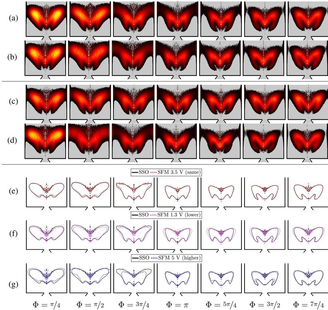
Figure 3.2. (a-d) Phase-averaged, Abel-transformed flame images shown in false colors. Light intensity of \text{OH}^* chemiluminescence is obtained at different phase instants of the acoustic cycle using an intensified camera. (a) Images obtained under SSO at a frequency f_0 = 533 Hz. I'_{\text{OH}^*}/\overline{I_{\text{OH}^*}} = 28.9\% . (b-d) Images corresponding to SFM at the frequency of SSO. (b) The forcing amplitude matches that observed during SSO ( I'_{\text{OH}^*}/\overline{I_{\text{OH}^*}} = 30.4\% ). (c) The forcing amplitude is lower than that observed during SSO ( I'_{\text{OH}^*}/\overline{I_{\text{OH}^*}} = 14.2\% ). (d) The forcing amplitude exceeds that observed during SSO ( I'_{\text{OH}^*}/\overline{I_{\text{OH}^*}} = 37.8\% ). (e-g) Flame isocontours determined by Otsu thresholding method for SSO (solid black line in (e-g)) and three levels of SFM (same—red dotted line in (e), lower—magenta dotted line in (f), and higher—blue dotted line in (g)) fluctuation level compared to SSO.
