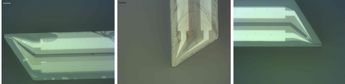
Figure 5.7: First set of shSQUIDs measured after they were RIEed and some of them FIBed. The clearest parts is the Al mask, the darker grey is the W layer. Even darker grey (all around Al masks in the left and right images) is the Si wafer. The size of each image is 120 \times 90 \mu\text{m}^2 .
