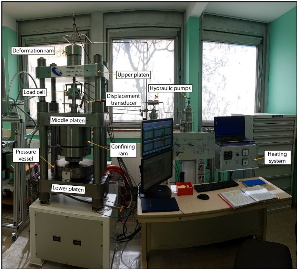
Figure III.7 : The new-Griggs apparatus installed at ISTO. From (Mansard, 2019).
